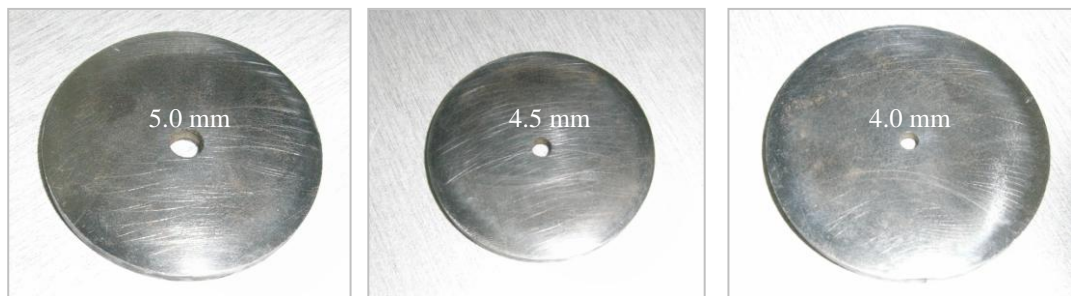
Figure 3.4: Fixed orifice plate with size of 4.0 mm, 4.5 mm and 5.0 mm
