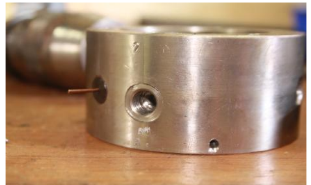
b) Copper pin installed
