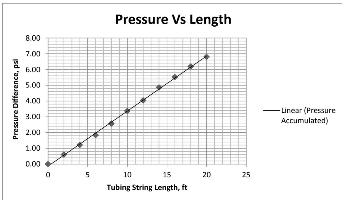
Figure 7 : Pressure Difference vs Tubing Length ( $Q_0=2000$  bbl/day)
