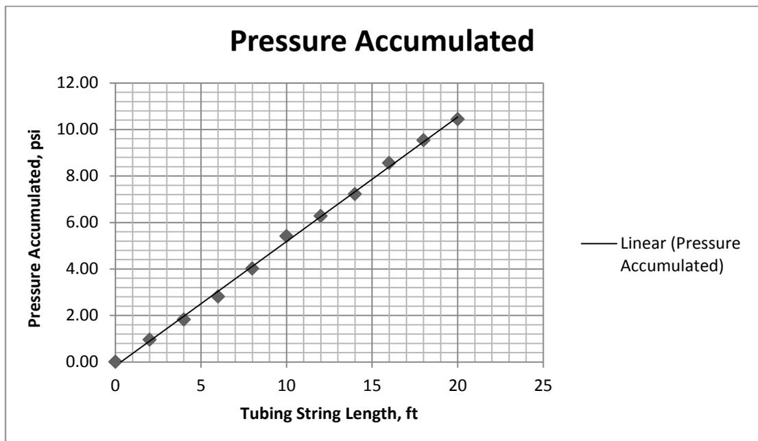
Figure 10 : Pressure Difference vs Tubing Length ( $Q_0= 3500$  bbl/day)
