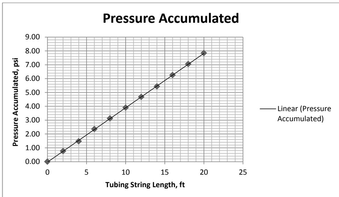
Figure 8 : Pressure Difference vs Tubing Length ( $Q_0 = 2500$  bbl/day)
