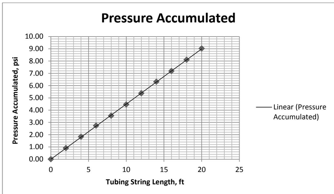
Figure 9 : Pressure Difference vs Tubing Length ( $Q_0 = 3000$  bbl/day)
