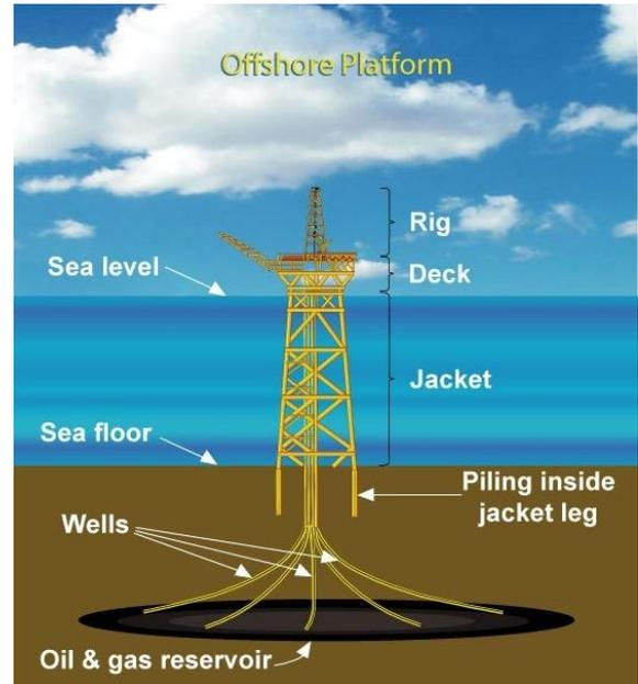
Figure 1: Example of an oil rig
