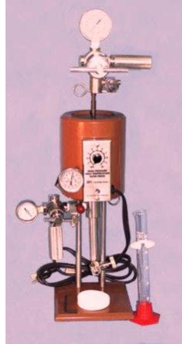
Figure 12 HPHT Filter Press Unit
