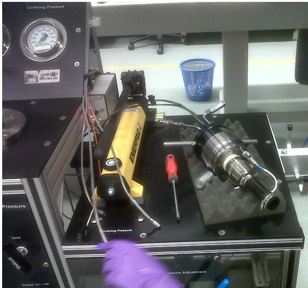
Figure 10 - Autolab Head (Transducers, Rubber Sleeve)
