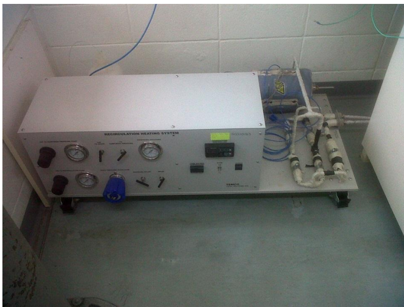
Figure 14 - NMR Cooling Unit
