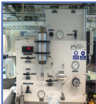
Figure 9: Benchtop Permeability System
