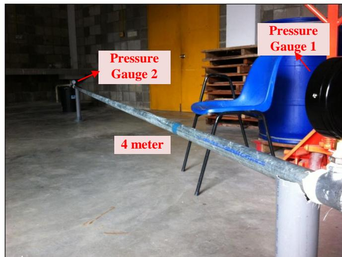
Figure 17: First pressure gauge to second pressure gauge
