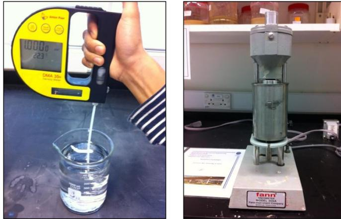
Figure 19: Digital density and Fann Viscometer
