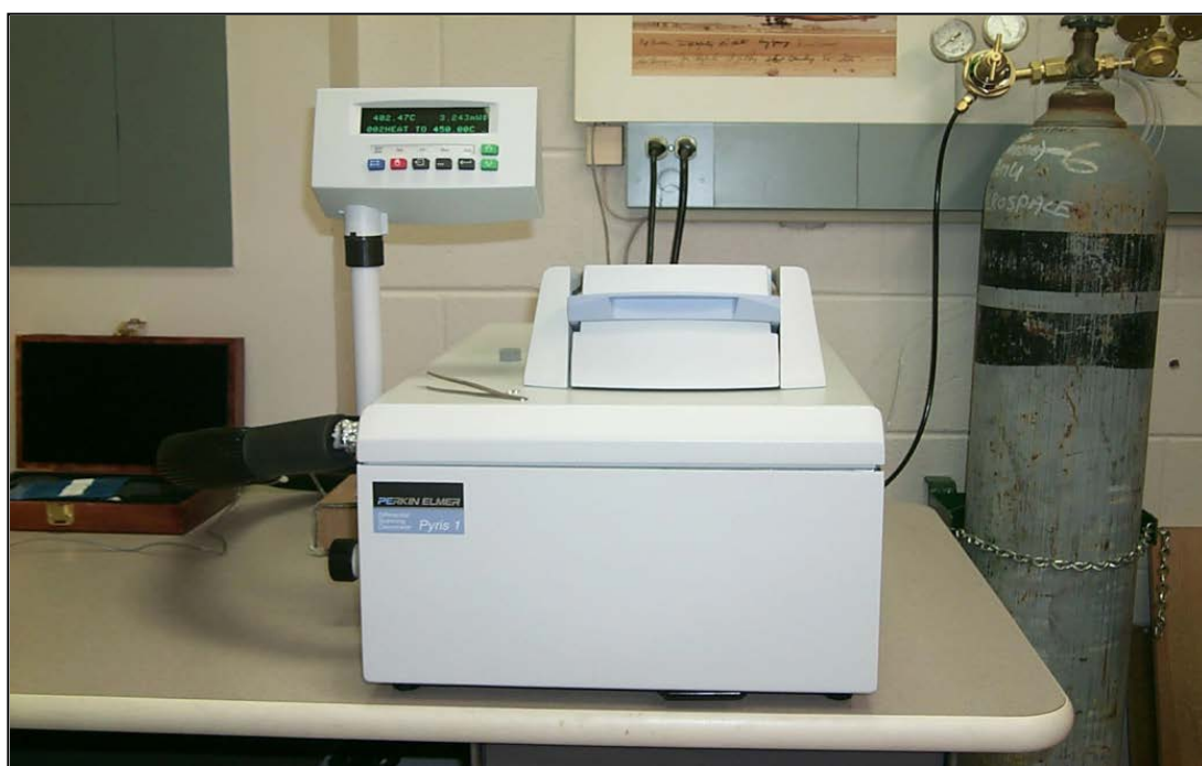
Figure 15: DSC equipment that will be used to investigate methane hydrate formation growth
