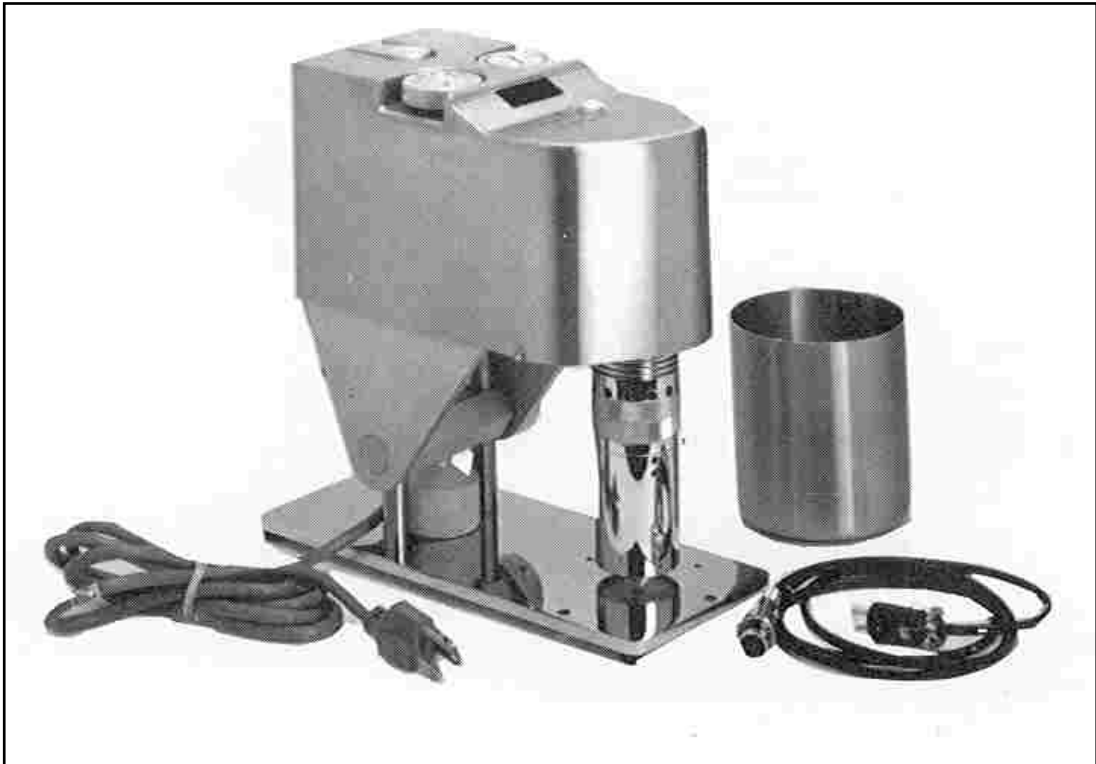
Figure 18: Rheometer that is used to studied PVP solution rheology
