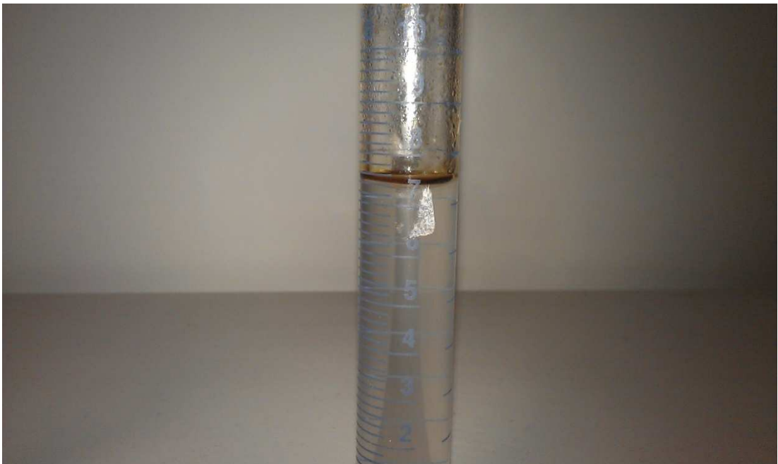
Figure 10: One of measuring tube which used to collect effluent during polymer flood at 90°C.
