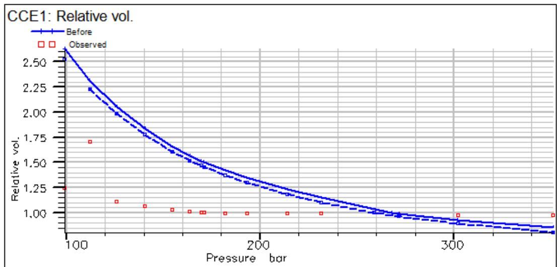
Figure 4.7: Comparison of regression result by tuning of  $P_c$  using SRK model
