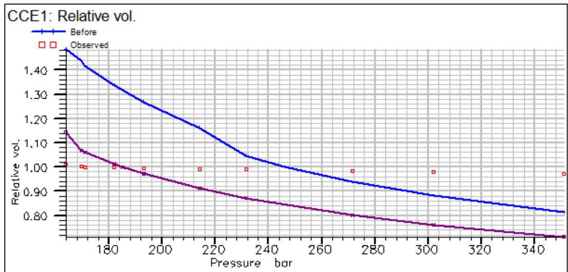
Figure 4.2: Comparison of regression result by tuning of  $T_c$  using PR model
