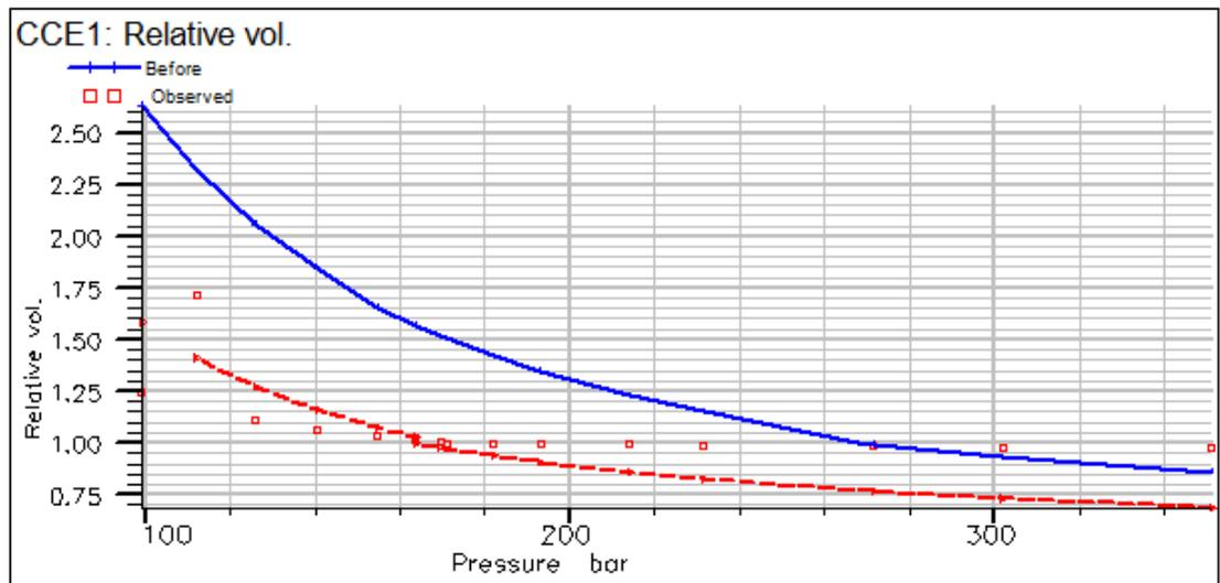
Figure 4.6: Comparison of regression result by tuning of  $T_c$  using SRK model
