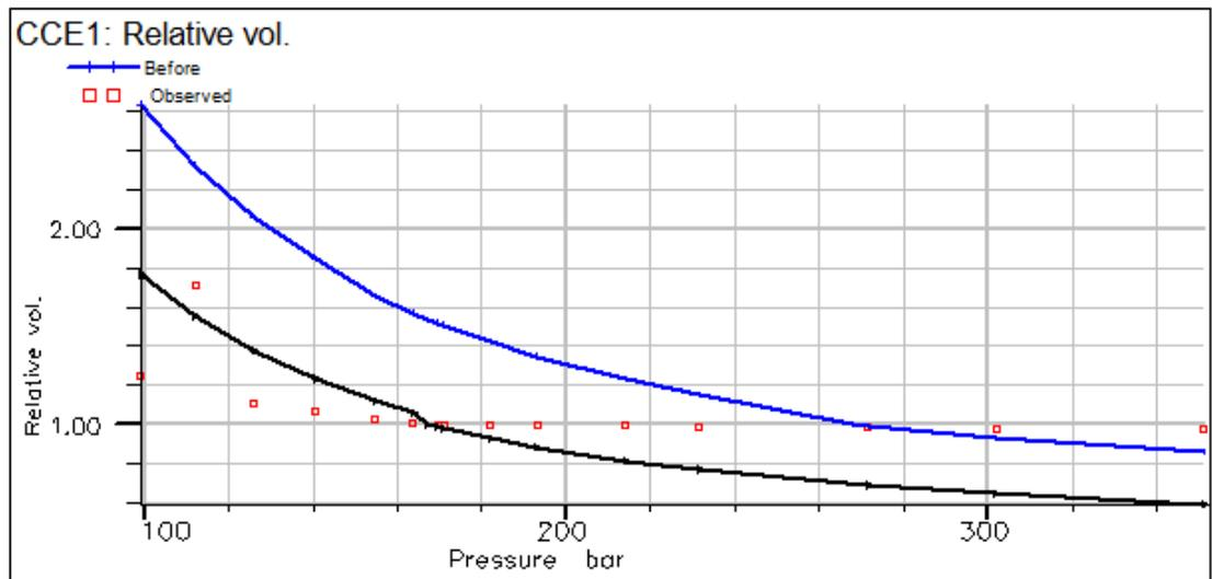
Figure 4.8: Comparison of regression result by tuning of AF using SRK model
