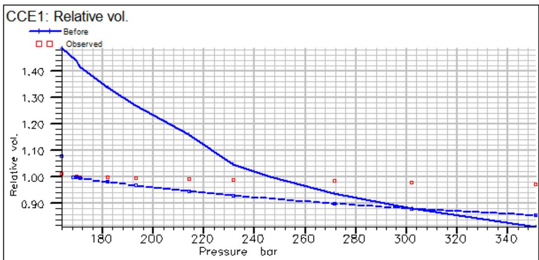
Figure 4.1: Comparison of regression result by tuning of all three variables using PR model
