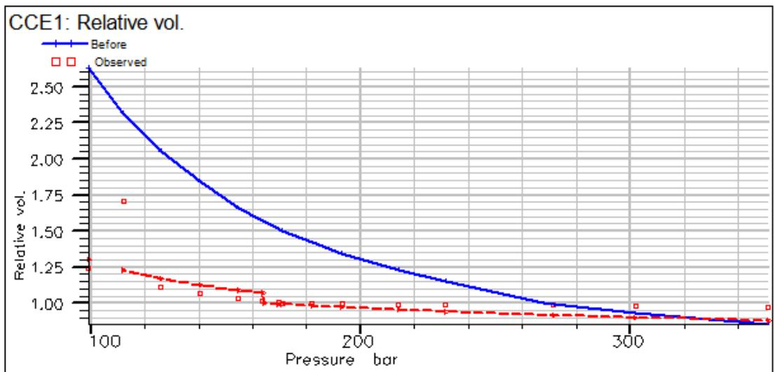
Figure 4.5: Comparison of regression result by tuning of all three variables using SRK model
