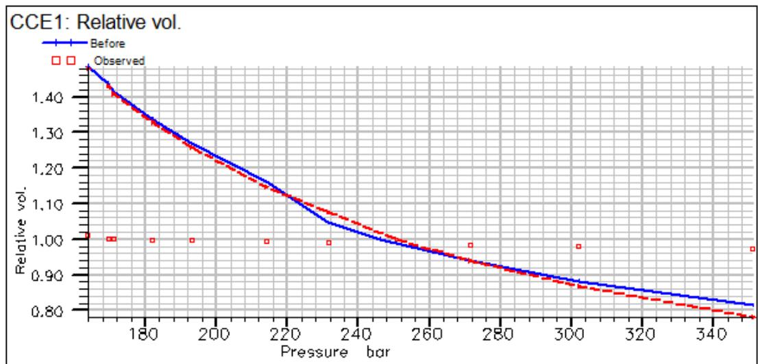
Figure 4.3: Comparison of regression result by tuning of  $P_c$  using PR model
