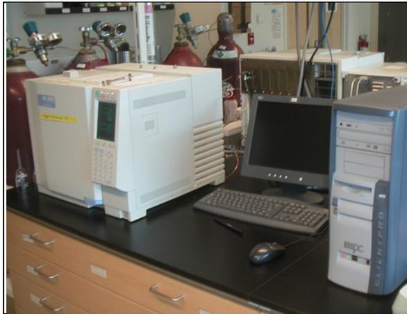
Figure 17: Shimadzu Gas Chromatograph GC-2010
