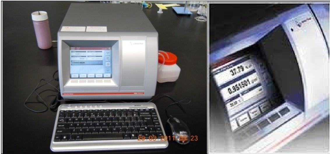
Figure 14: Anton Paar Density Meter 4500 M
