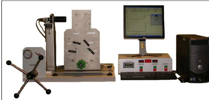
Figure 15: VINCI Technologies Interfacial Tensometer IFT 700
