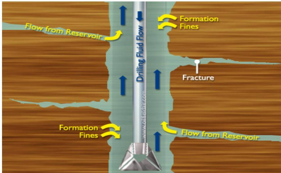
Figure 2: Underbalanced Drilling (Rigzone, 2011)
