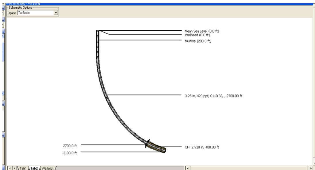
Figure 6: Design of the Studied Well by using Landmark Compass
