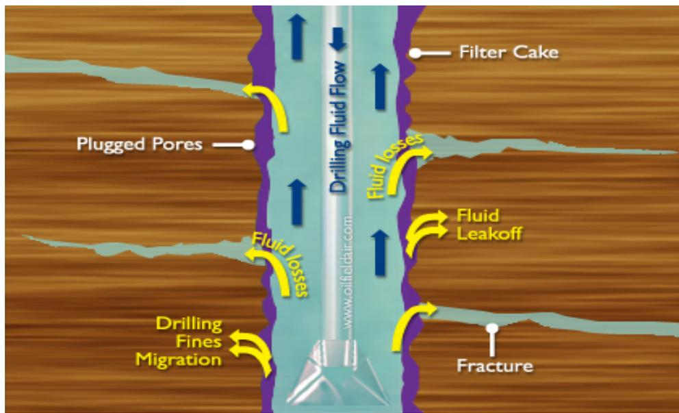
Figure 1: Conventional Drilling (Rigzone, 2011)
