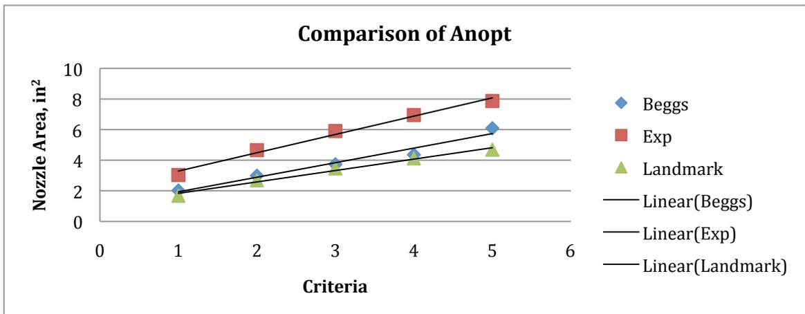
Figure 11: Comparison Graph of  $A_{nopt}$  between Criteria of 3 Methods
