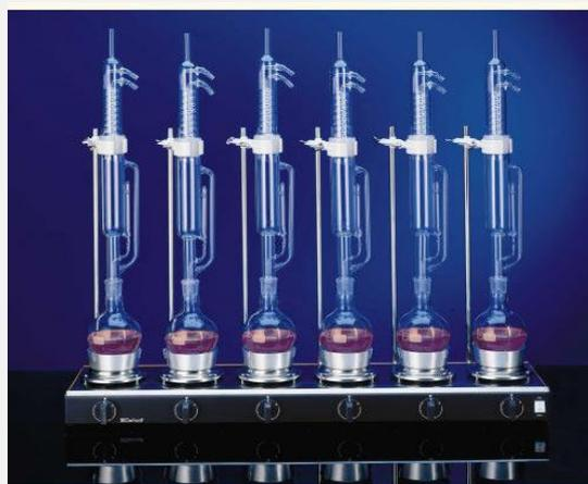
Figure 8: Soxhlet Extractor
