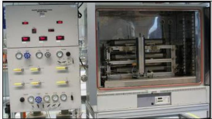
Figure 6: Relative Permeability Test System
