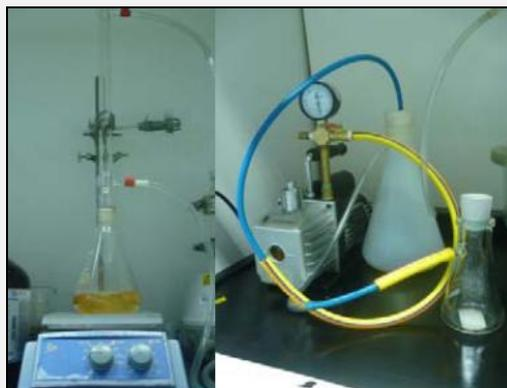
Figure 5: ASTM D3279-07 Standard Test Method for n-Heptane
