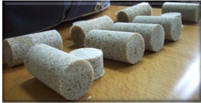
Figure-6: The cores after being drilled to a size of 1.5” diameter and 2” long
