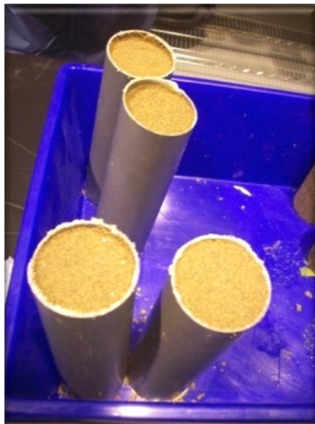
Figure-3 : Sand preparation into core in PVC pipes
