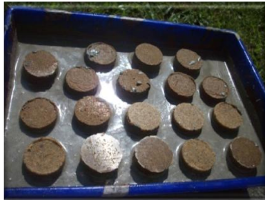
Figure-5: The cores are cemented in a rectangle plastic container
