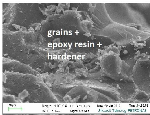
Figure 15: Sample-9 before acid saturation
