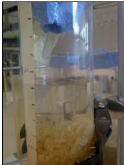
Figure 4.6 Water Ponding in Bioretention Column
