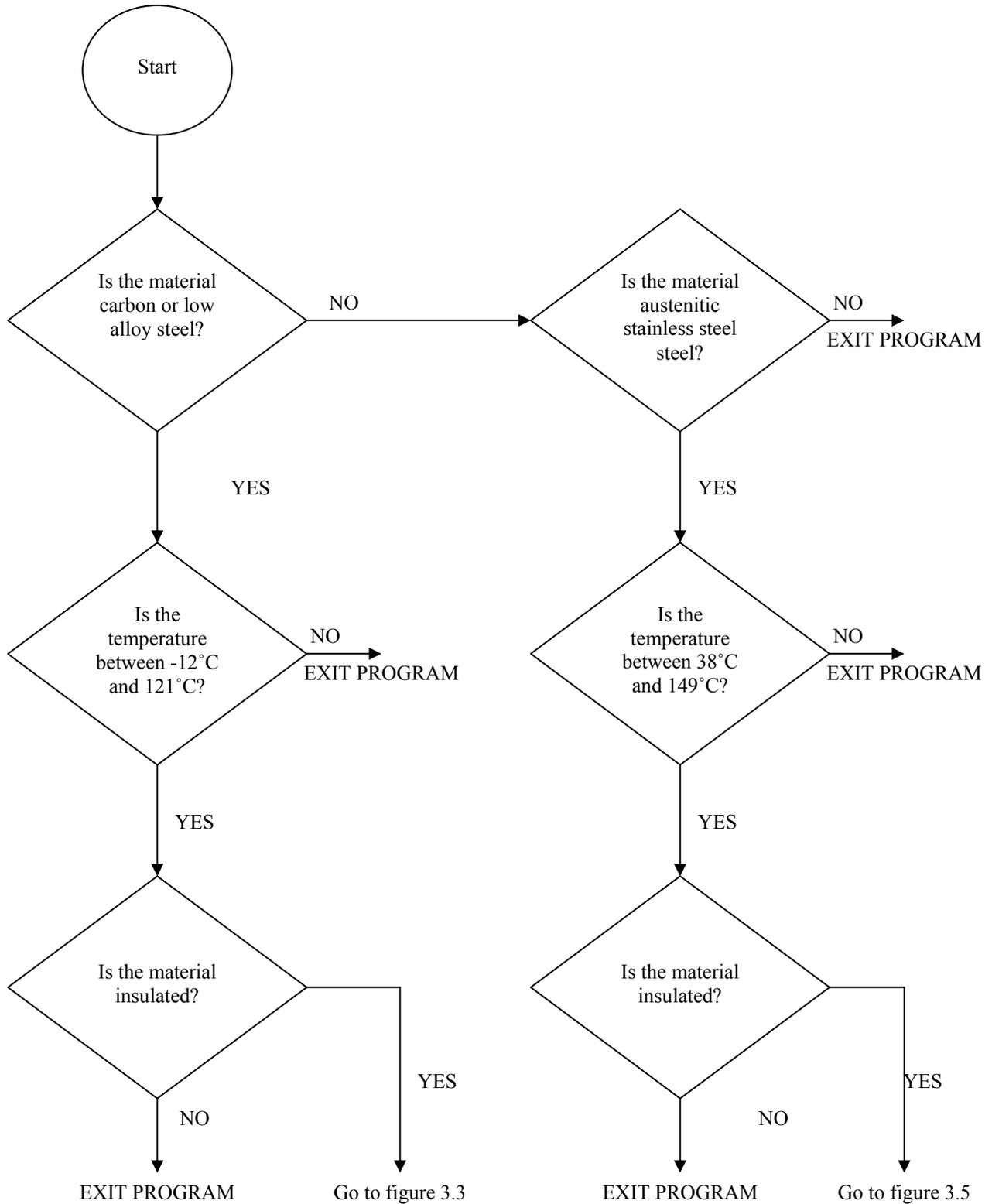
Figure 3.2: Flowchart for External Damage [9]
