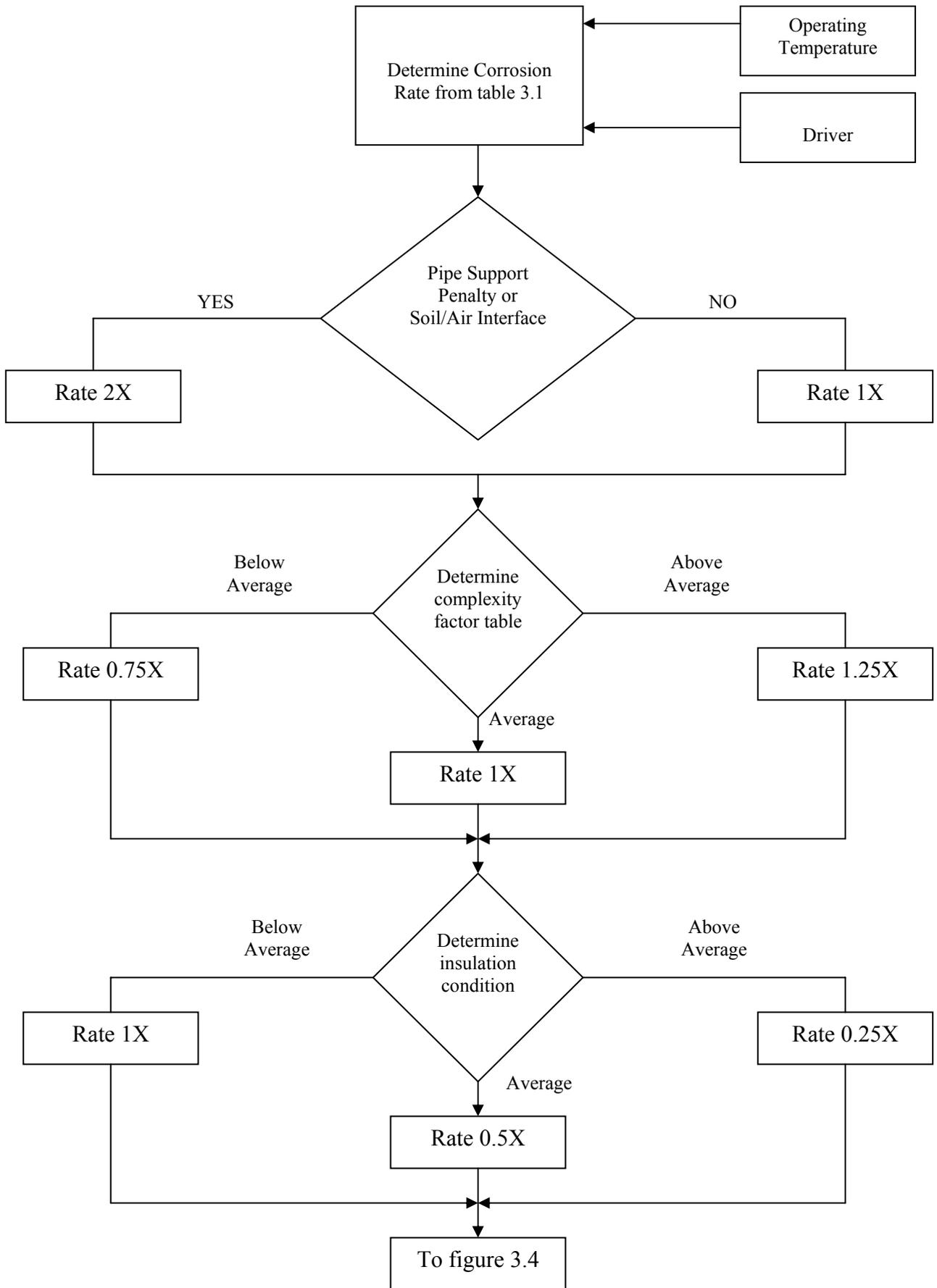
Figure 3.3: Flowchart of CUI for Carbon Steel [9]
