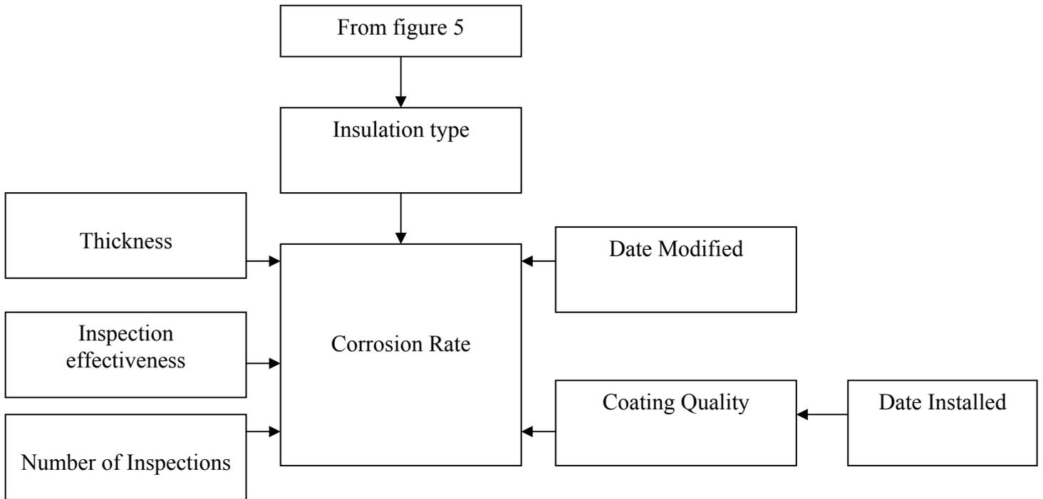
Figure 3.6: Flowchart of External CUI SCC for Austenitic Stainless Steels (cont) [9]
