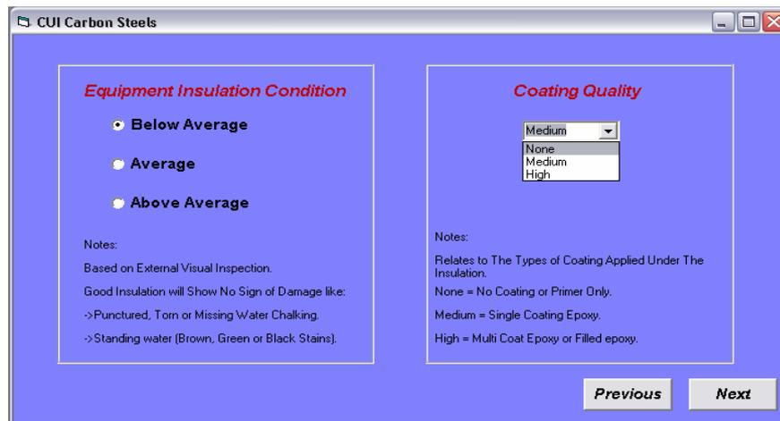
Figure 4.8: Interface to Determine Insulation Condition and Coating Quality
