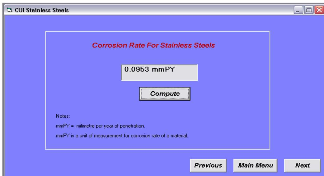
Figure 4.15: Interface to compute Corrosion Rate for Stainless Steels
