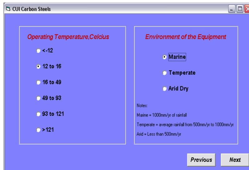
Figure 4.5: Interface to Determine Operating temperature and Environment
