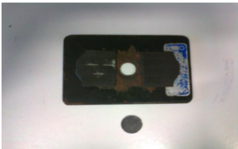
FTIR sample (after compression)
