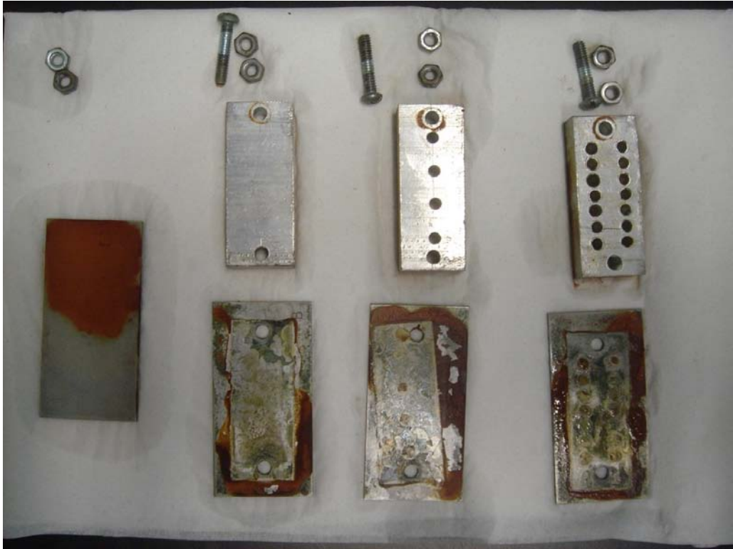
Figure 5.16: (From left) Control Specimen, Sacrificial Anodes D, E and F after 14 days
