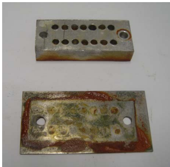
Figure 5.19: Sacrificial Anode F after 14 days
