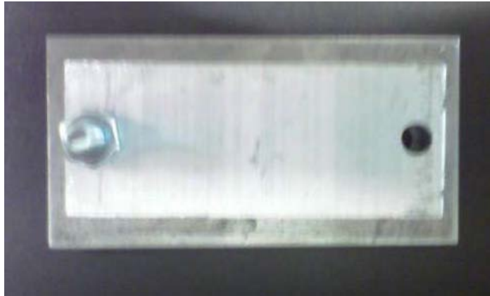
Figure 5.5: Sacrificial Anode D being stacked on Steel Plate
