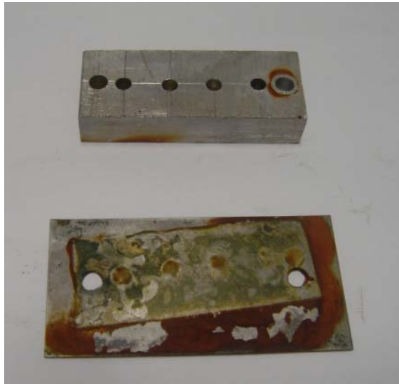
Figure 5.18: Sacrificial Anode E after 14 days
