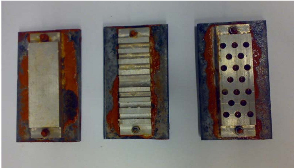
Figure 5.15: (From left) Sacrificial Anodes D, E and F after 14 days
