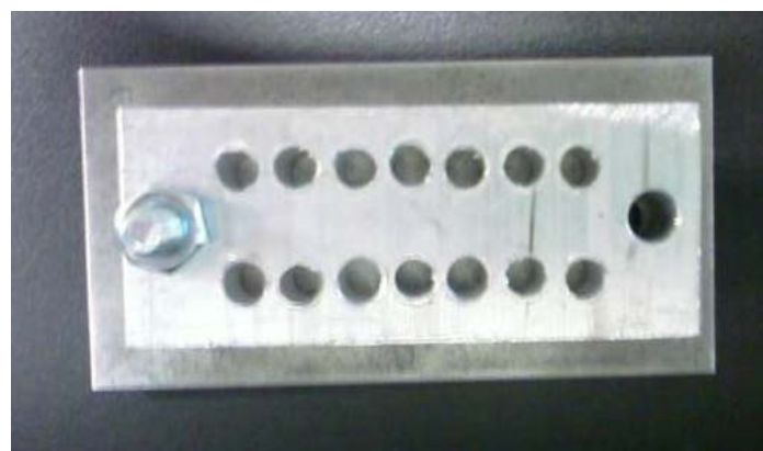
Figure 5.7: Sacrificial Anode F being stacked on Steel Plate
