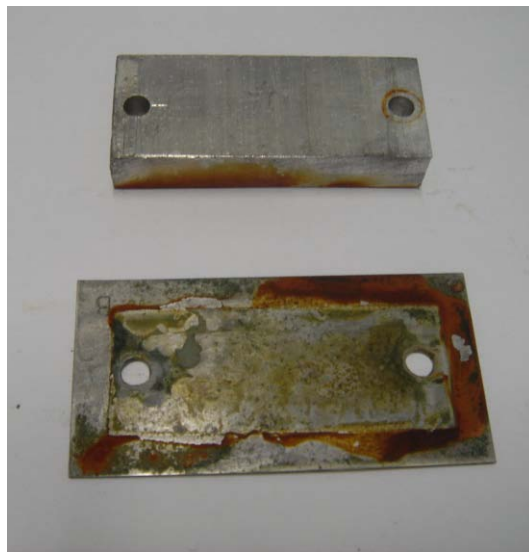
Figure 5.17: Sacrificial Anode D after 14 days
