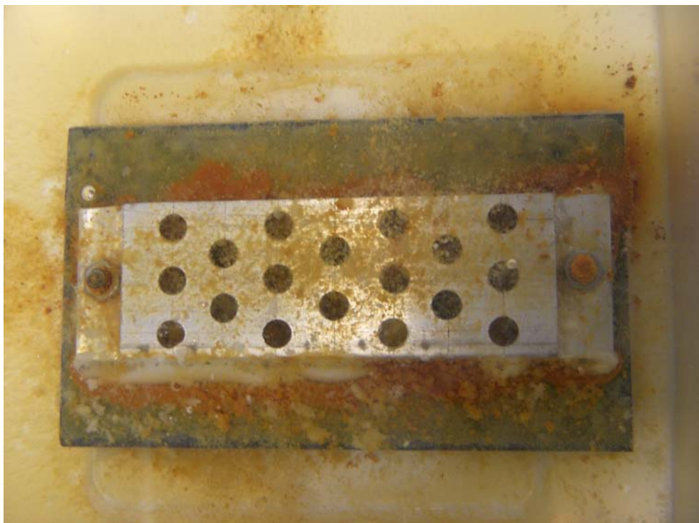
Figure 5.13: Sacrificial Anode C after 7 days (Sample 3)
