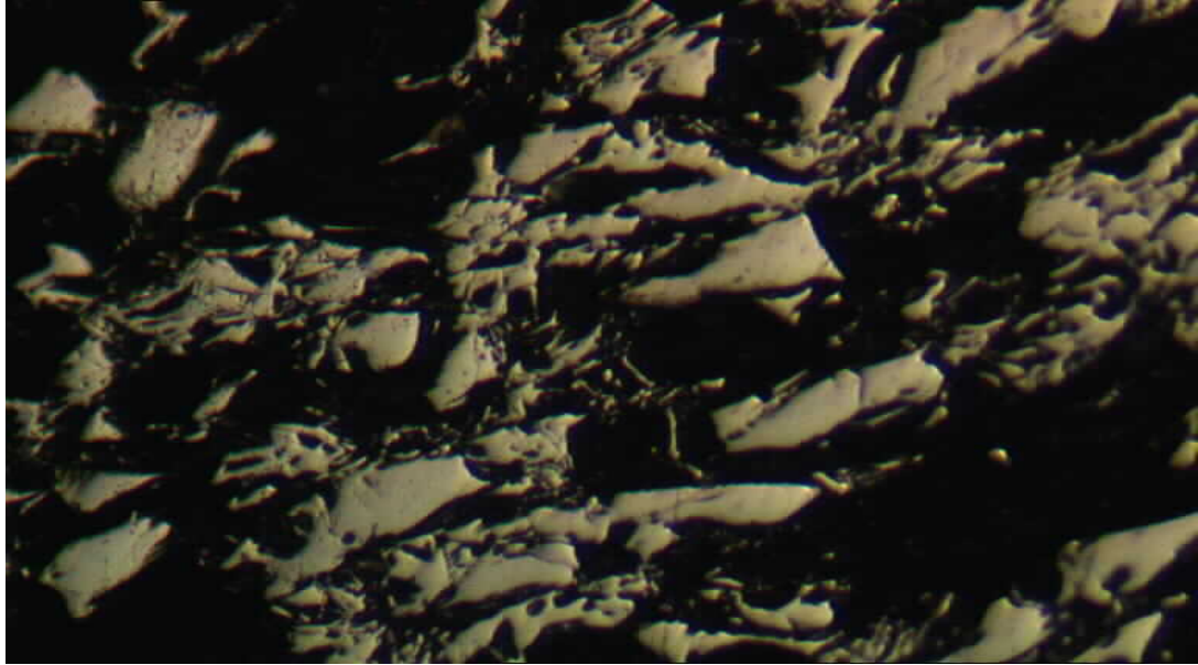
Figure 4.7: Optical microscope image of the NdFeB Magnet
