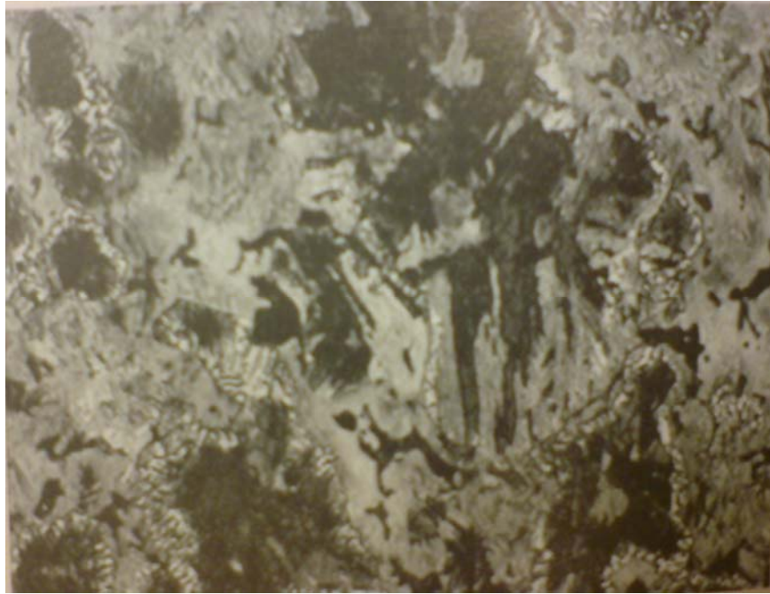
Figure 2.4: FLN4-4405 extra fine Ni powder [4]
