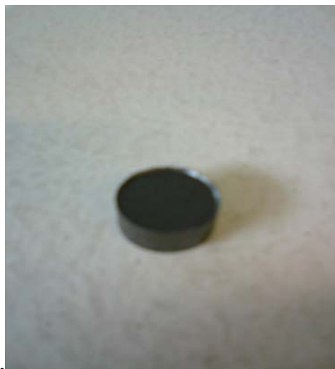
Figure 4.10: Compacted powder (green compact) in pallet form
