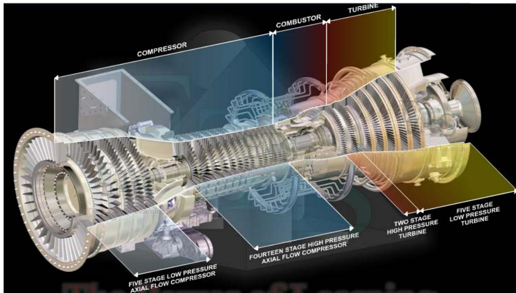
**Figure 1.3:** Industrial gas turbine layout [4]
