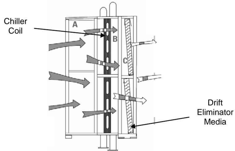
**Figure 2.7:** Chiller system mechanism [7]
