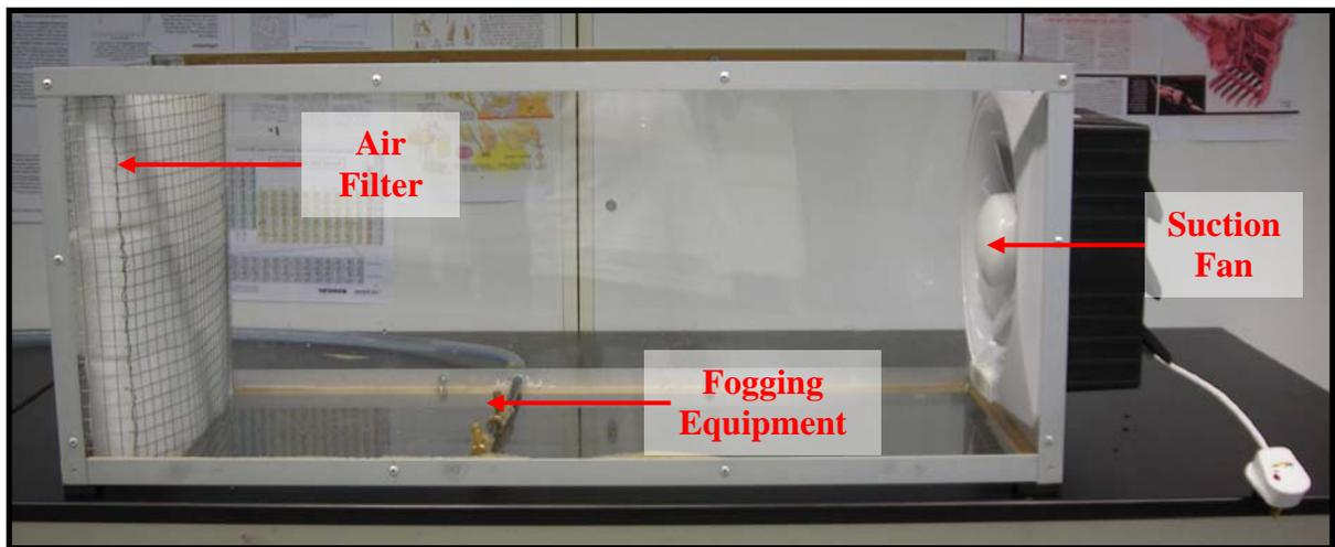
**Figure 3.3:** Prototype of the cooler system
