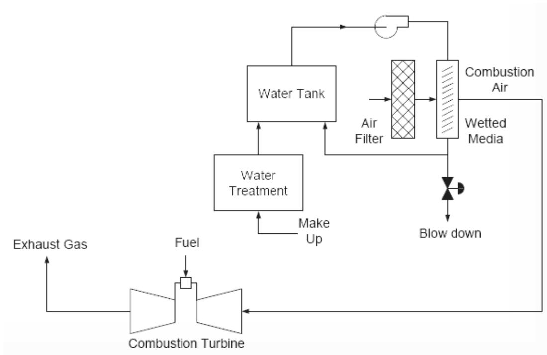
**Figure 2.6:** Schematic of evaporative media cooling [7]
