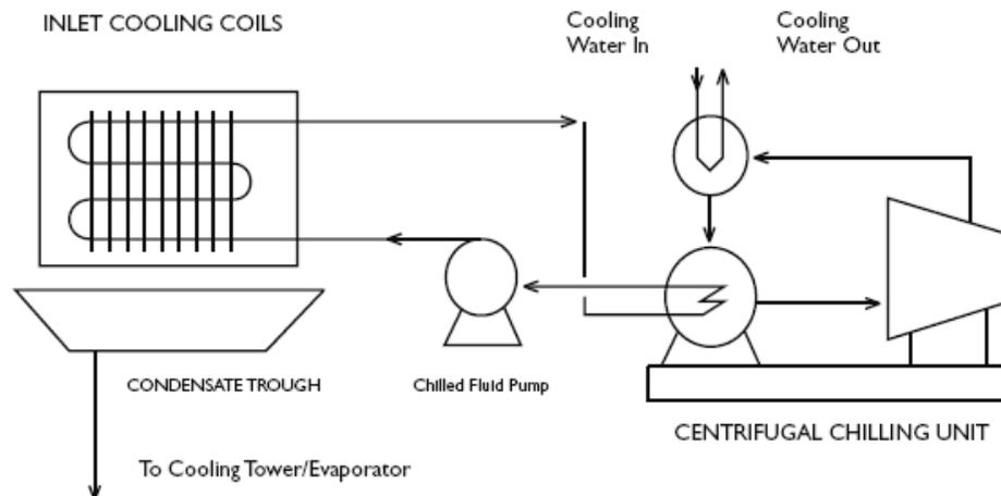
**Figure 2.8:** Schematic diagram of a chiller system [7]
