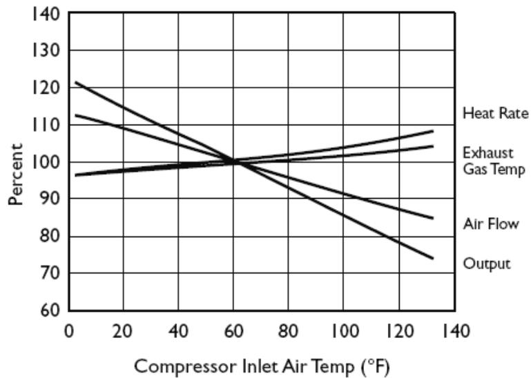
**Figure 2.2:** Effect of compressor air inlet temperature on gas turbine performance [6]
