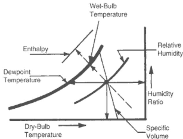
**Figure 4.3:** Properties of moist air on a psychrometric chart
