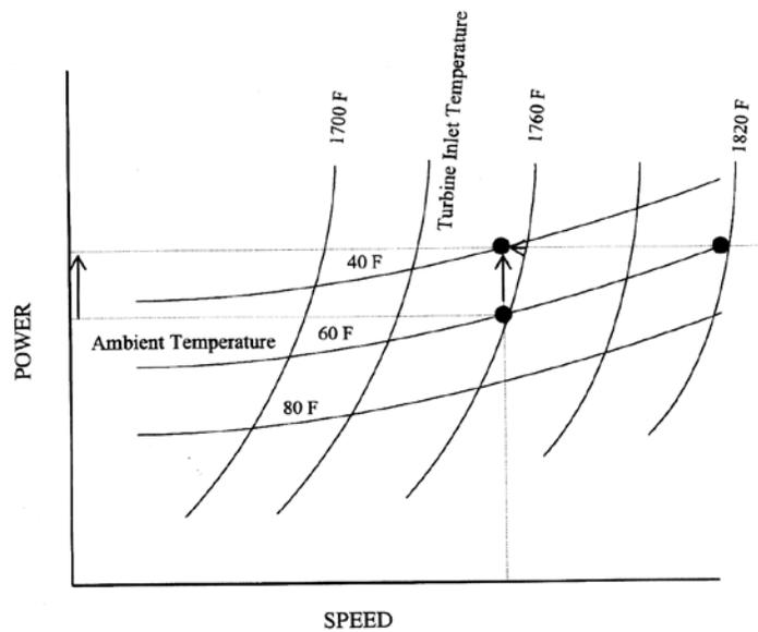
**Figure 2.1:** Temperature-power-speed interrelationships [5]
