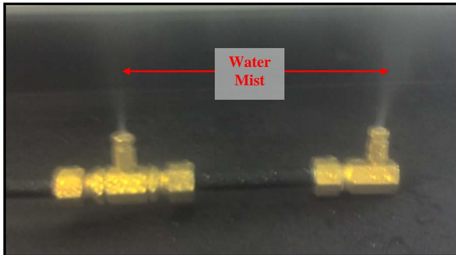
**Figure 3.7:** Atomization of nozzles
