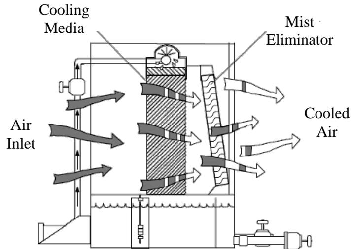
**Figure 2.5:** Evaporative media cooling mechanism [7]
