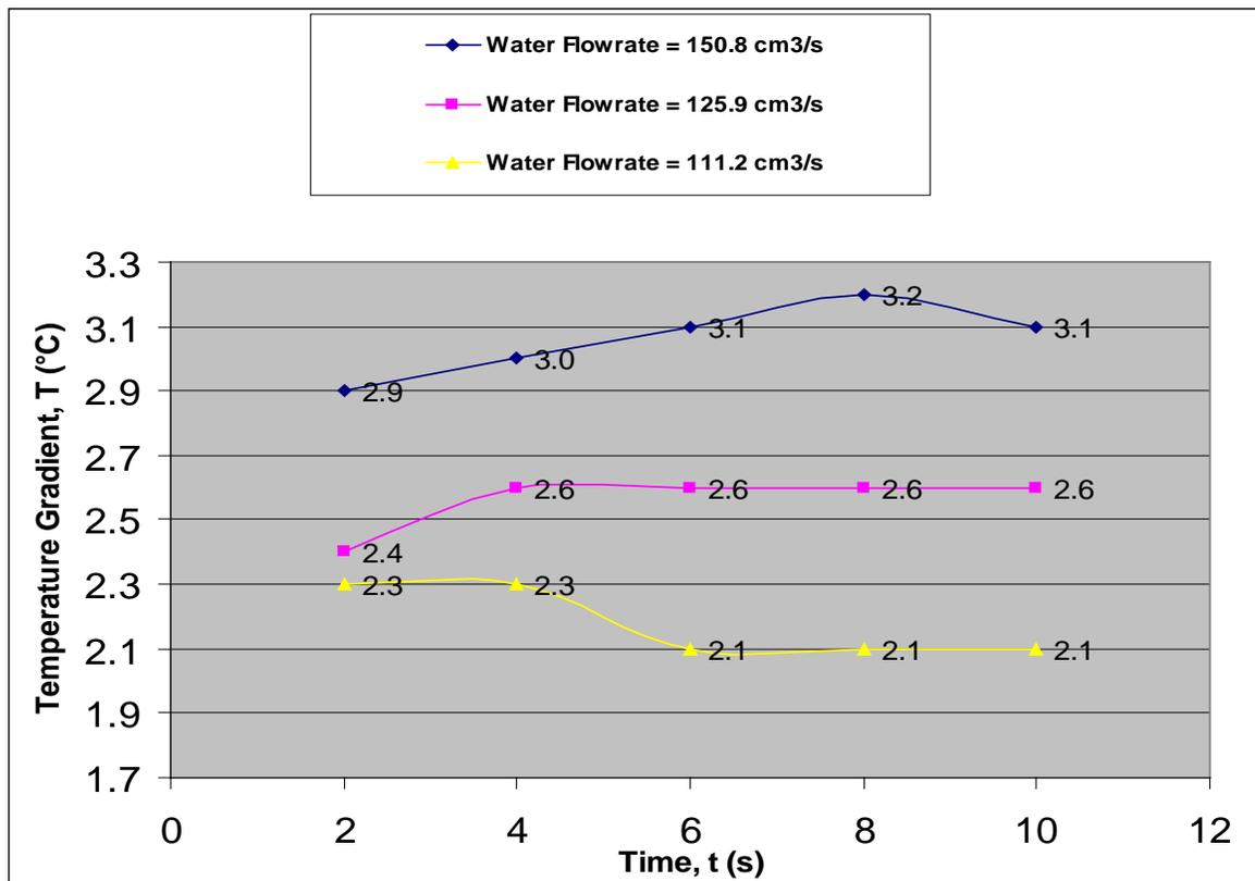
**Figure 4.4:** Graph temperature gradient vs. time with different water flowrate
