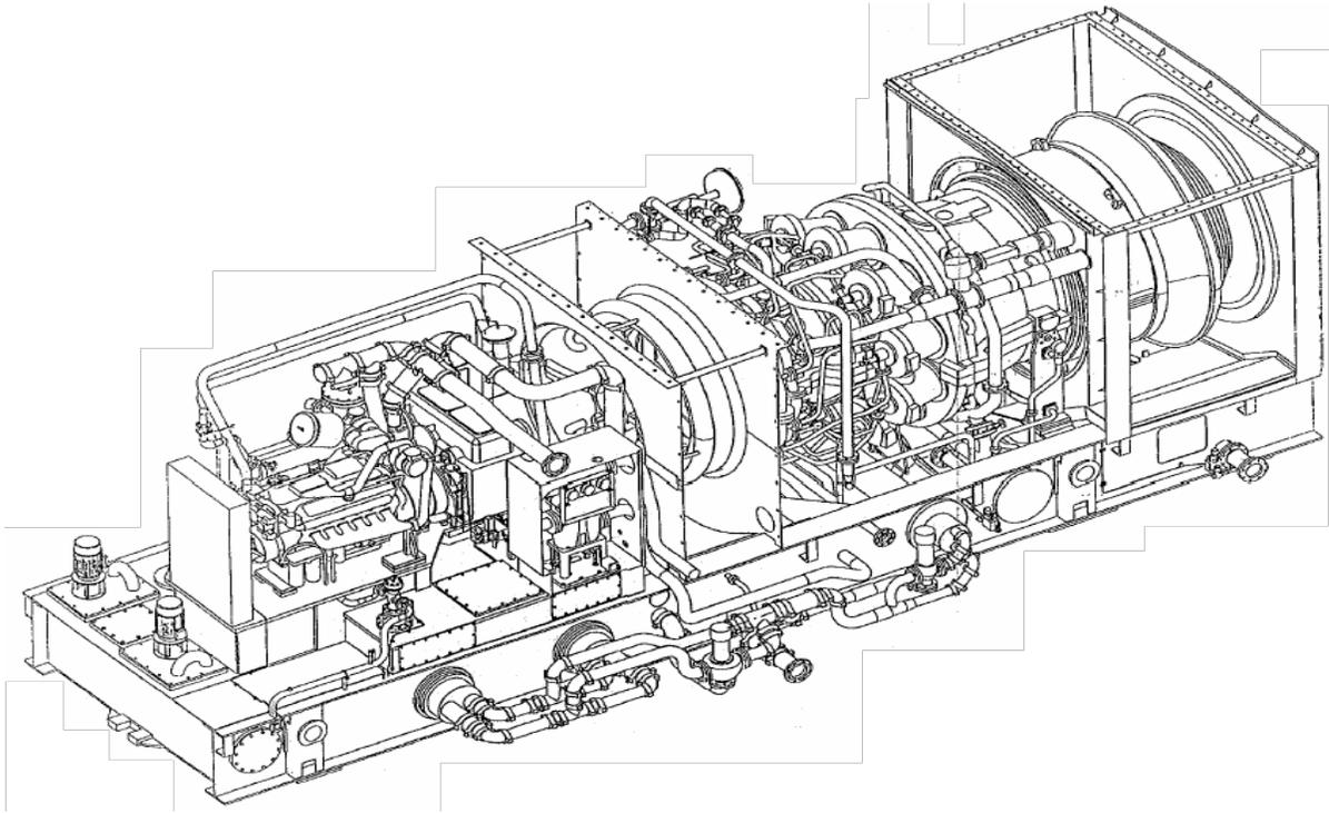
**Figure 4.1:** Layout of GE MS6001B gas turbine used at CUF
