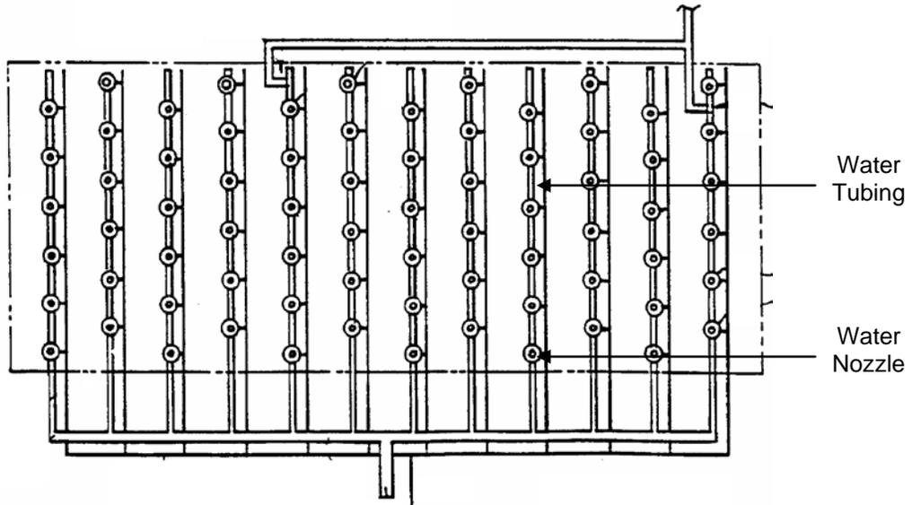
**Figure 2.10:** Plan View of an array of fogging system [8]
