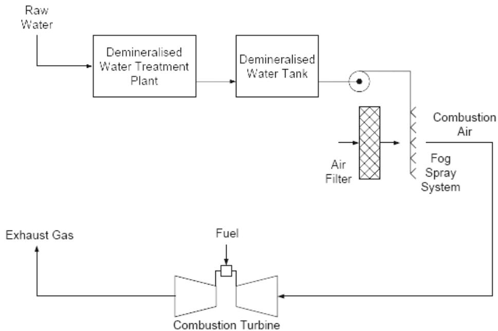
**Figure 2.4:** Schematic diagram for fogging system [7]
