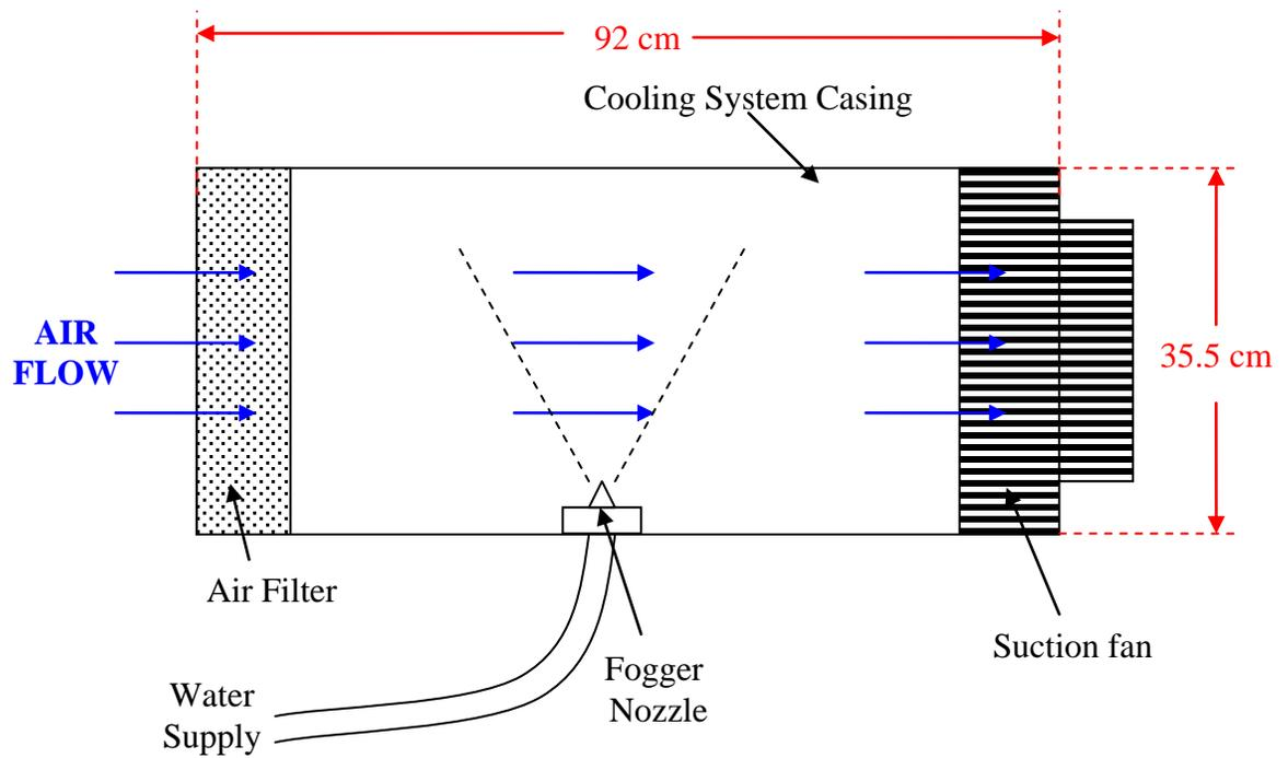
Figure 3.1: 2-D model of the prototype
