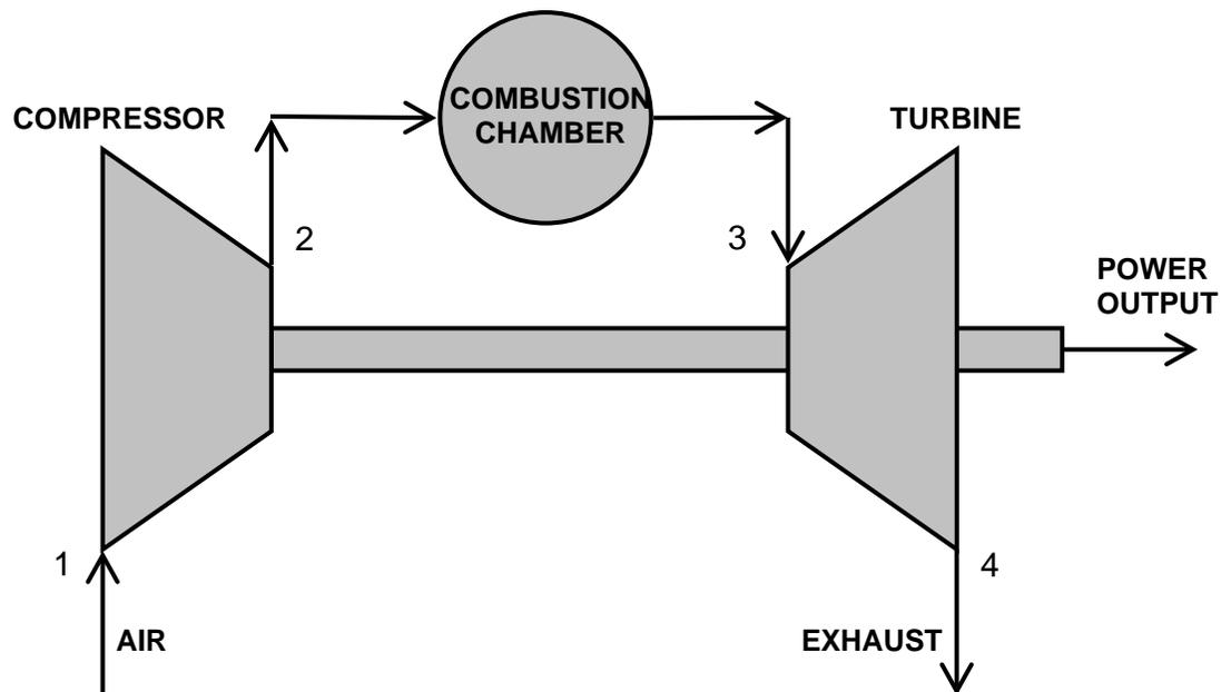
**Figure 1.1:** Gas turbine cycle
