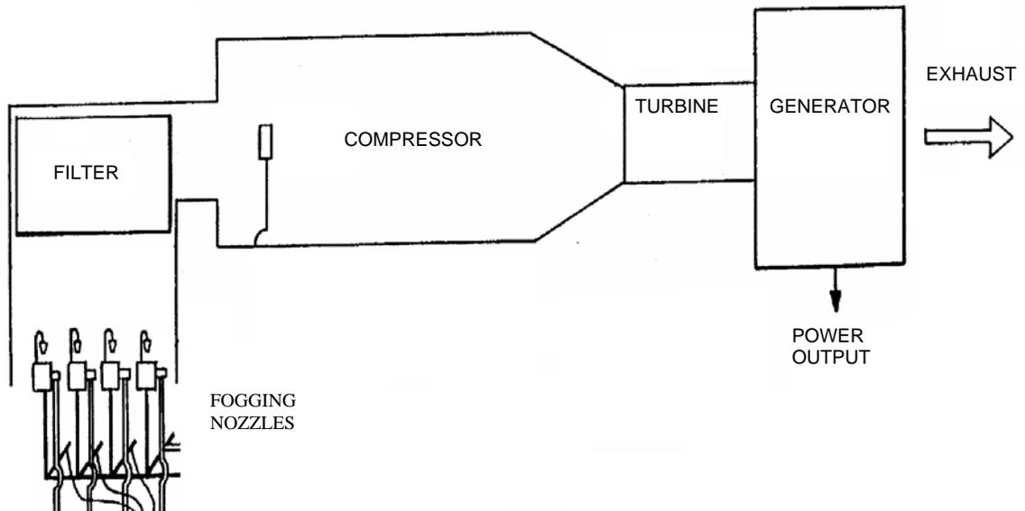
**Figure 2.9:** Application of fogging system in gas turbine [8]
