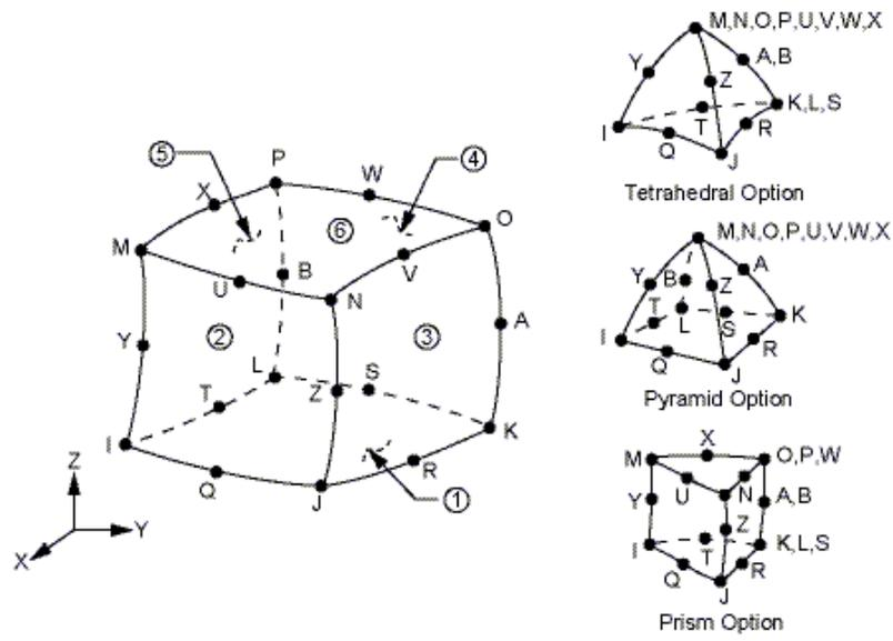
**Figure 2.10:** "SOLID90 Geometry"
