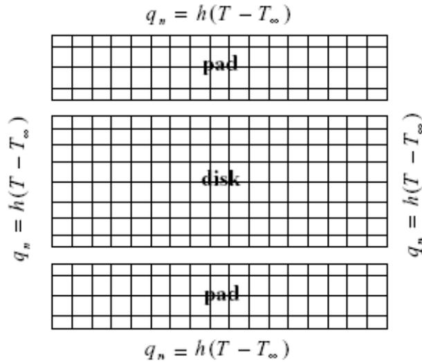
**Figure 2.9:** Heat finite element models for the transient temperature analysis
