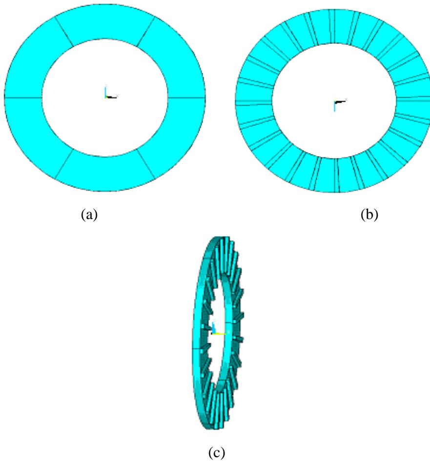
**Figure 3.5:** Picture of disc volume modelling in ANSYS, (a) Top View, (b) Bottom View, (c) Isometric View
