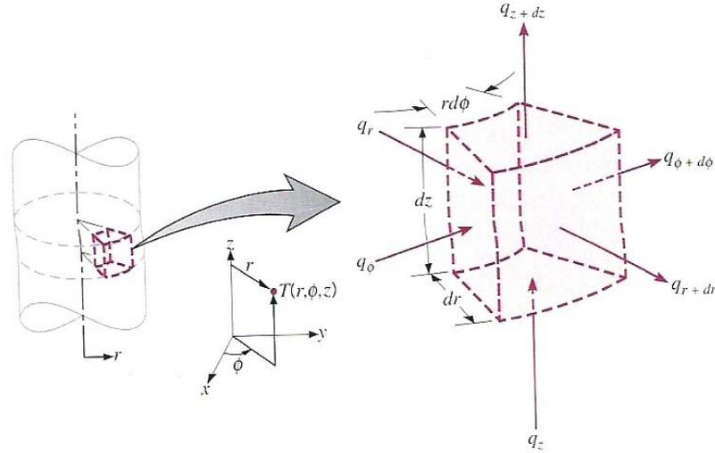
**Figure 2.7:** Differential control volume for conduction analysis in Cylindrical coordinates
