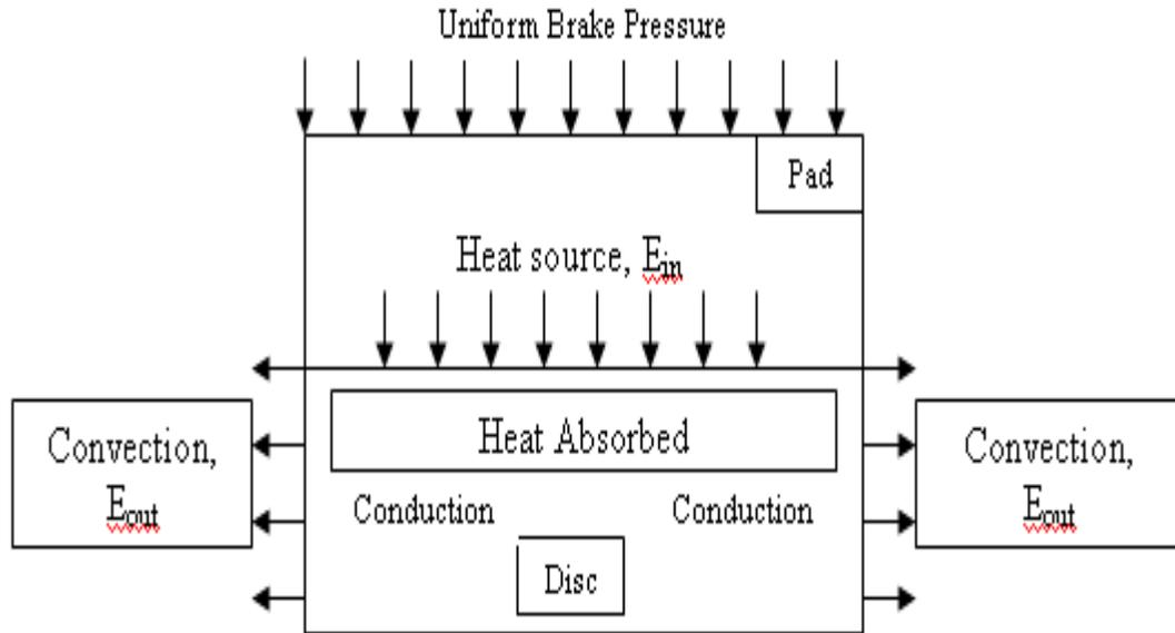
**Figure 2.1:** Heat balance in a brake disc during the brake application
