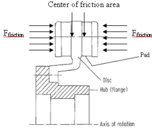
**Figure 2.5:** Axle layout of disc brake when Brake force applied
