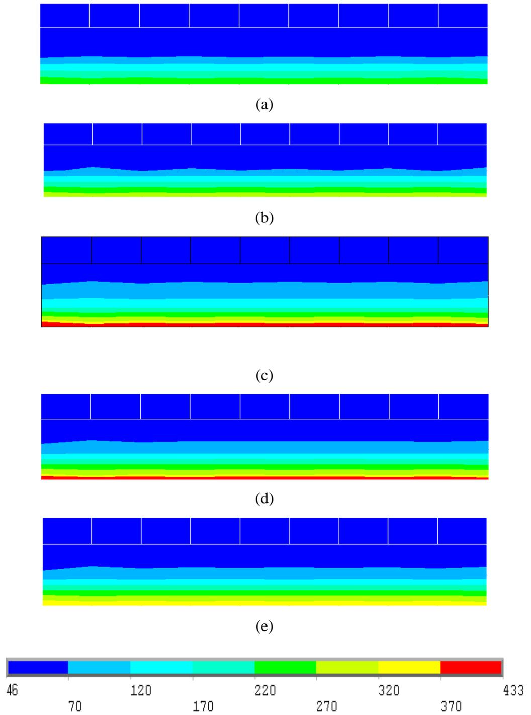
**Figure 4.12:** Surface temperature contours at (a) 0.1415s, (b) 0.2878s, (c) 2.5476s, (d) 3.0497s and (e) 3.9472 s
