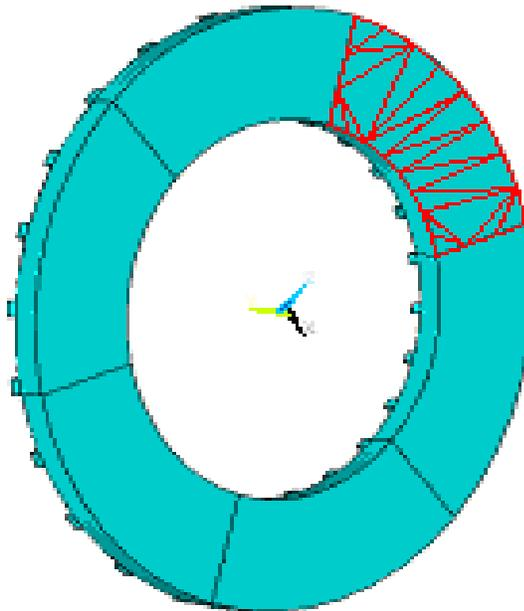
**Figure 3.6:** Sections highlighted represent pad contact area where heat flux is applied
