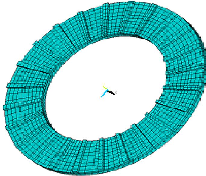
**Figure 3.7:** Mashed pattern on the surface volume of the disc brake
