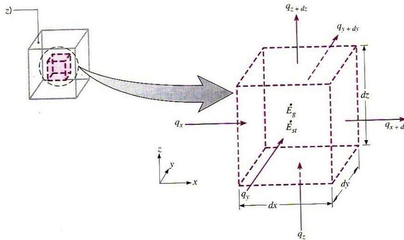
**Figure 2.6:** Differential control volume for conduction analysis in Cartesian Coordinates
