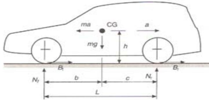
**Figure 2.2:** Free body diagram of a vehicle during braking
