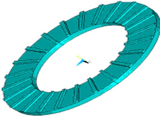
**Figure 3.4:** Three-dimensional model of disc brake with cutting sections of ventilated wall
