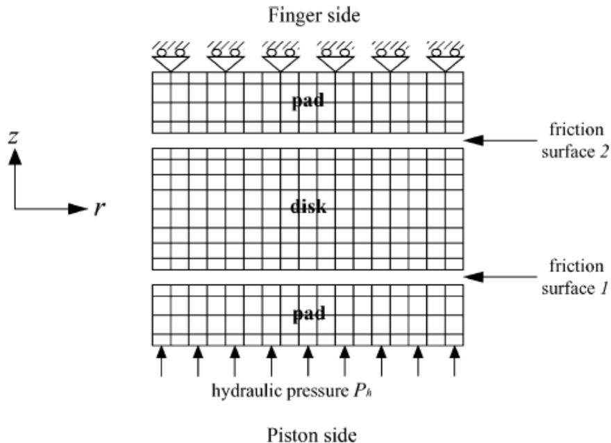
**Figure 2.8:** Finite element model for the transient temperature analysis
