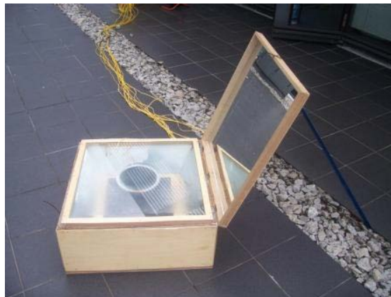
Figure 3.20 : Performance testing of a box type solar cooker.
