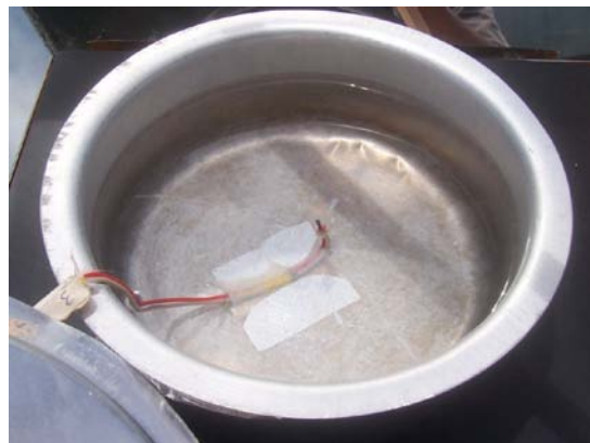
Figure 3.21 : Thermocouple is submerged in water inside the cooking pot.
