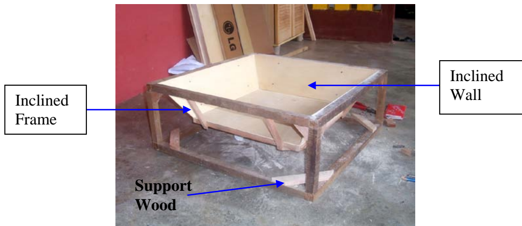
Figure 3.18 : Assembly of main frame with cooking chamber of solar cooker
