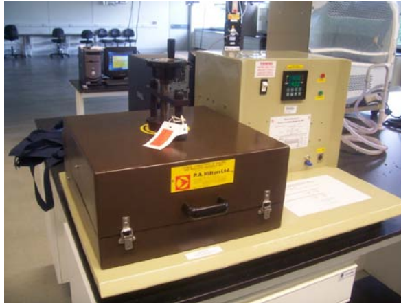
Figure 3.10 : Equipment used to determine thermal conductivity of materials
