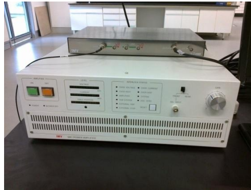
Figure 10: Controller for Vibration Shaker
