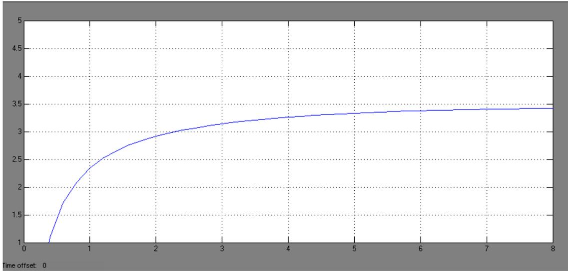
Figure 27 : Charging Curve with current value of 0.4A
