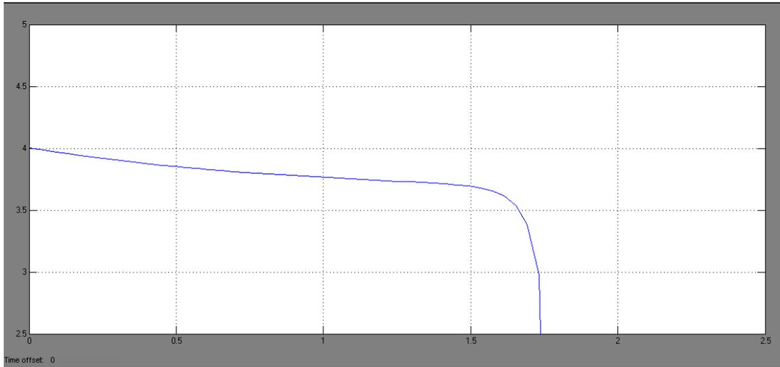
Figure 21 : Discharge Curve with SOC initial 0.89 (10 cycle time) with load 0.94 ohm
