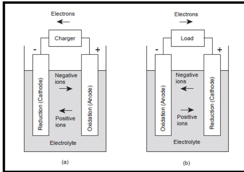
Figure 6 : Electrochemical operation of battery during charging (a) and discharging (b)
