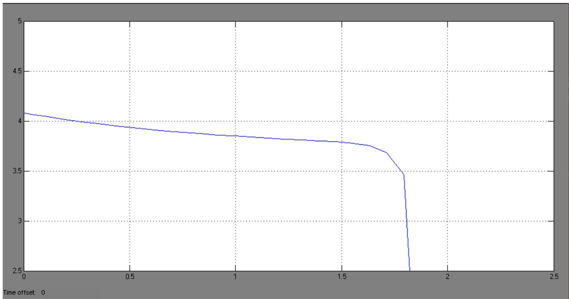
Figure 22 : Discharge Curve with SOC initial 0.89 (10 cycle time) with load 1.04 ohm
