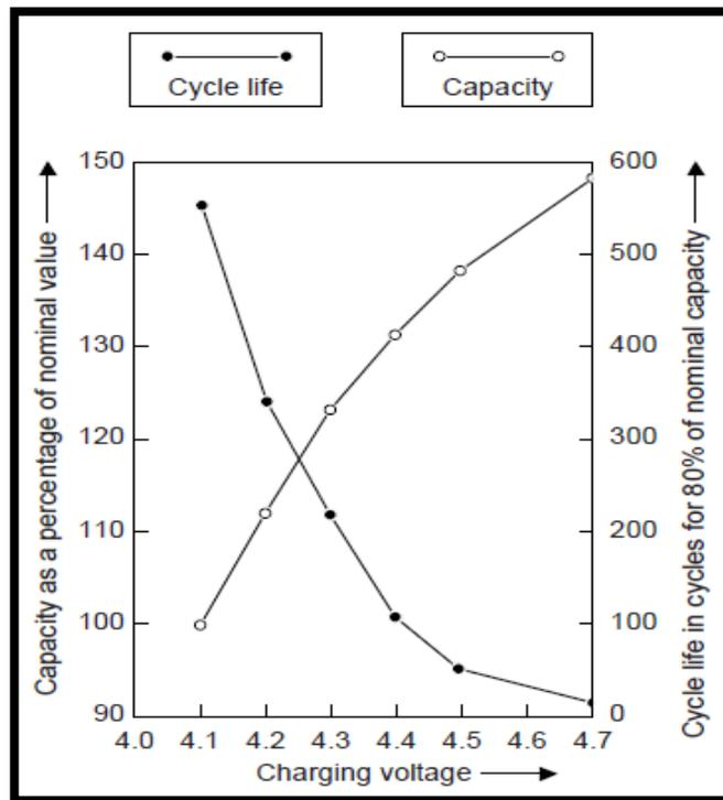
Figure 3: Maximum battery capacity and cycle life as a function of a battery voltage for Li-Ion Battery
