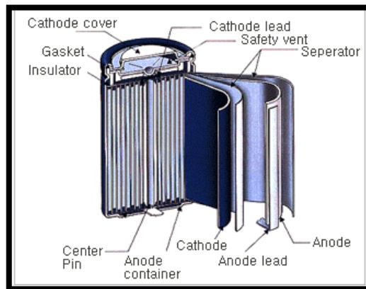
Figure 4 : Structure of Lithium-Ion Battery
