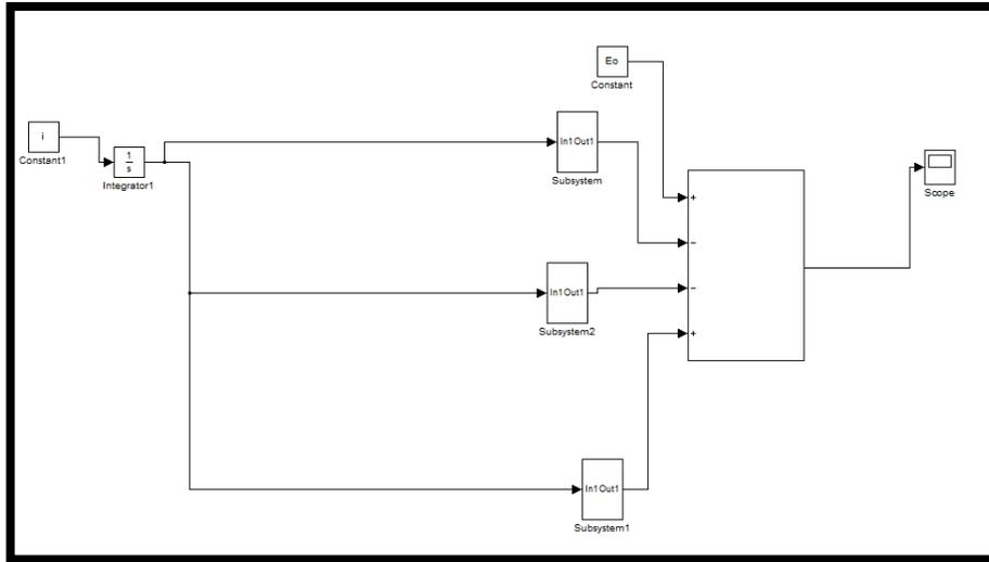
Figure 16 : Simulation Block Diagram of the Main System (Charging)
