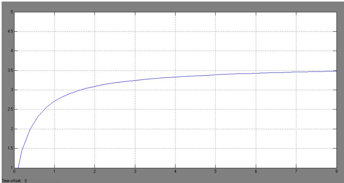
Figure 26 : Charging Curve with current value of 0.2A
