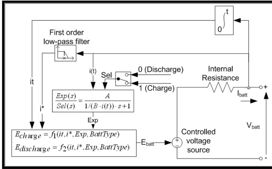
Figure 7 : Non- Linear Battery Model
