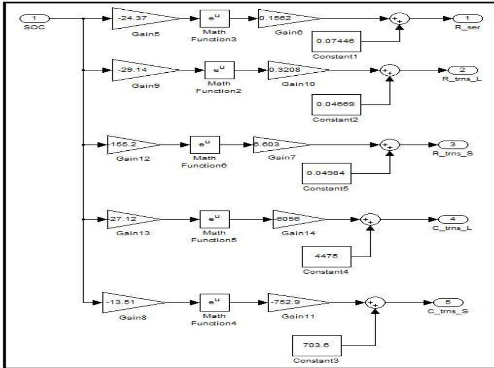
Figure 14: Simulation Block Diagram for Impedance
