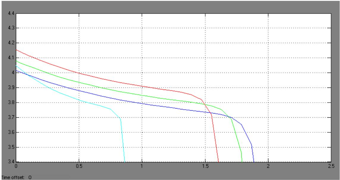
Figure 25 : Over-discharge curve (Line 4) due to heavy current supply
