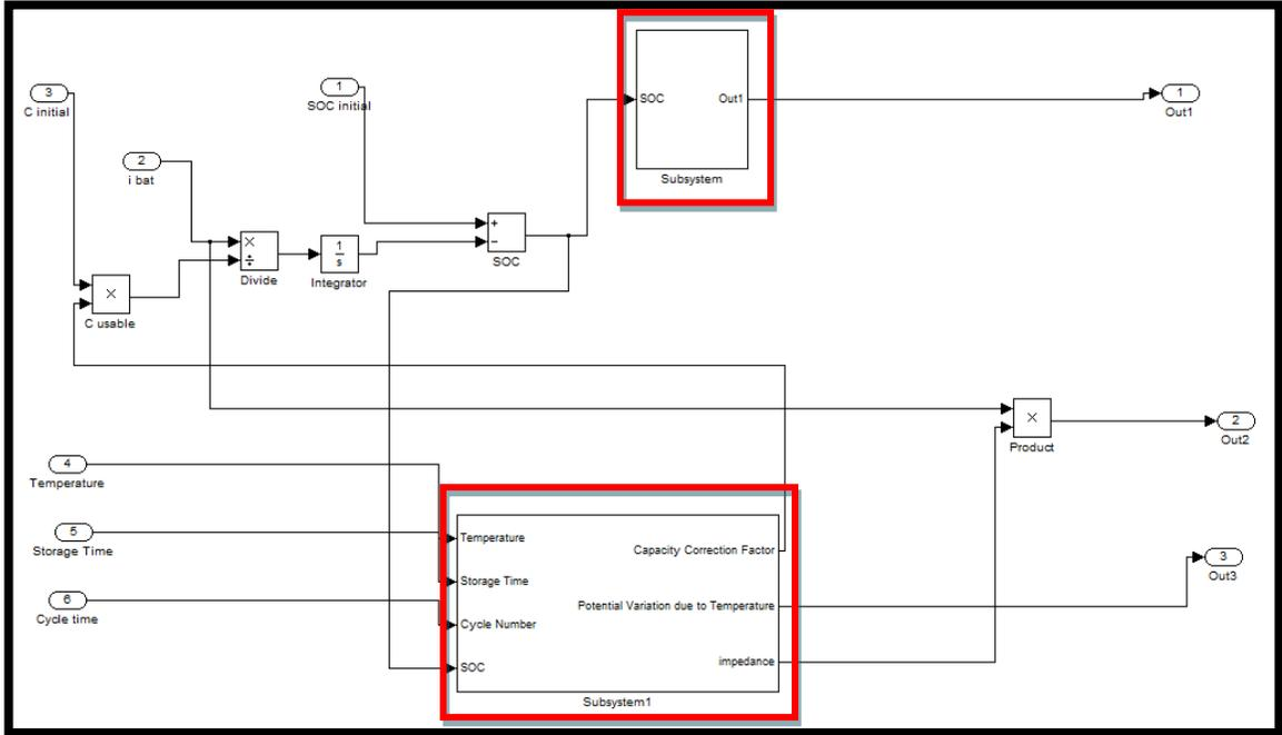
Figure 11 : Simulation Block Diagram for Voltage Open Circuit
