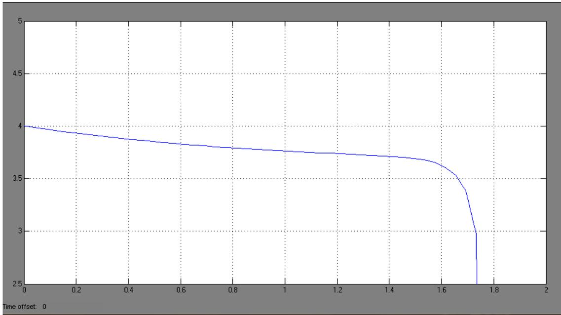
Figure 20 : Discharge Curve with SOC initial 0.89 (10 cycle time) & current value 0.9A
