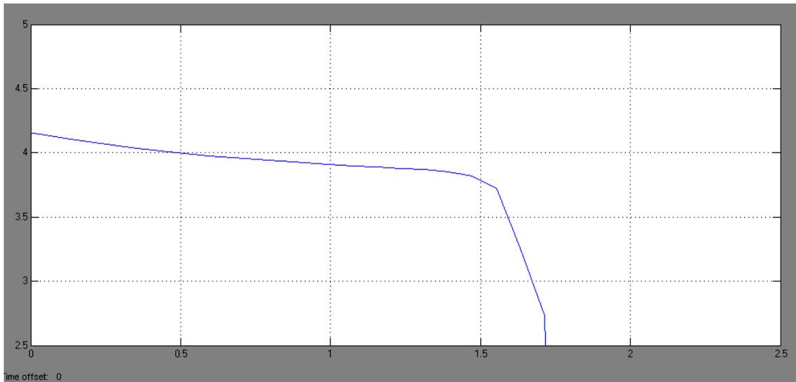
Figure 23: Discharge Curve with SOC initial 0.89 (10 cycle time) with load of 1.11 ohm
