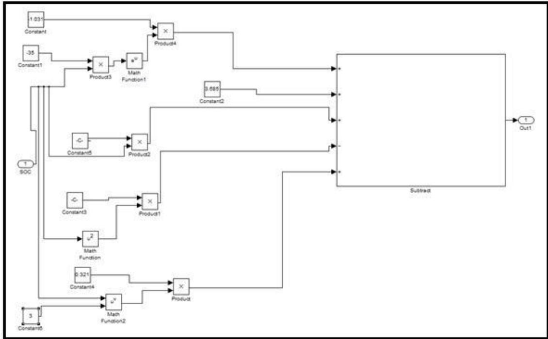
Figure 12 : Simulation Block Diagram for Voltage Open Circuit dependent in battery SOC (Subsystem)
