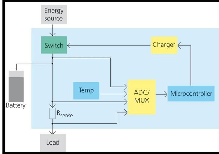
Figure 5 : General Architecture of a Battery Management System
