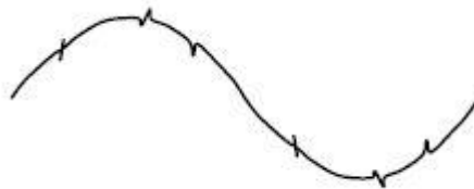
Figure 8: Waveform undergoing notching
