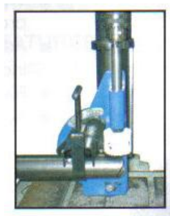
Figure 4-17 Typical pipe notcher (Anthony M O'Neill, 2005)
