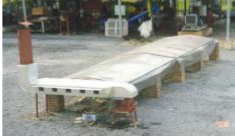
FIGURE 2.5: Solar-biomass Hybrid Tunnel Dryer [11]
