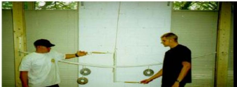
**Figure 3a:** Two students demonstrate moment in Lab. The “beam” is made out of PVC pipe. There are actually two PVC beams: one behind, to which a moment is being imparted by two hanging weights, and one in front, which is cut in half so that students can measure the amount of force required to duplicate the curve of the pipe behind it.
