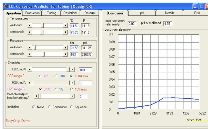
Figure 4.2.1.5: Corrosion rate monitoring at pure CO<sub>2</sub> condition.
