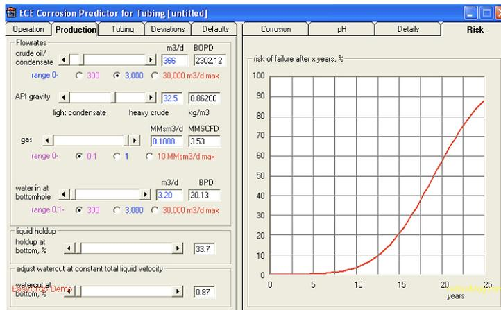
Figure 4.2.1.8: Failure risk increase with presence of water in gas producing wells.
