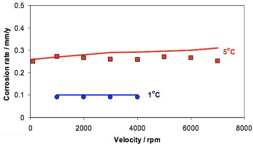
Figure 2.2.2: Comparison between experimental results (points) and predictions (line) for the new updated model at low temperature.
