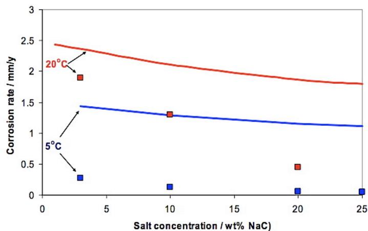
Figure 2.2.3: Comparison between experimental results (points) and predictions (lines) for the original model at various NaCl concentrations.
