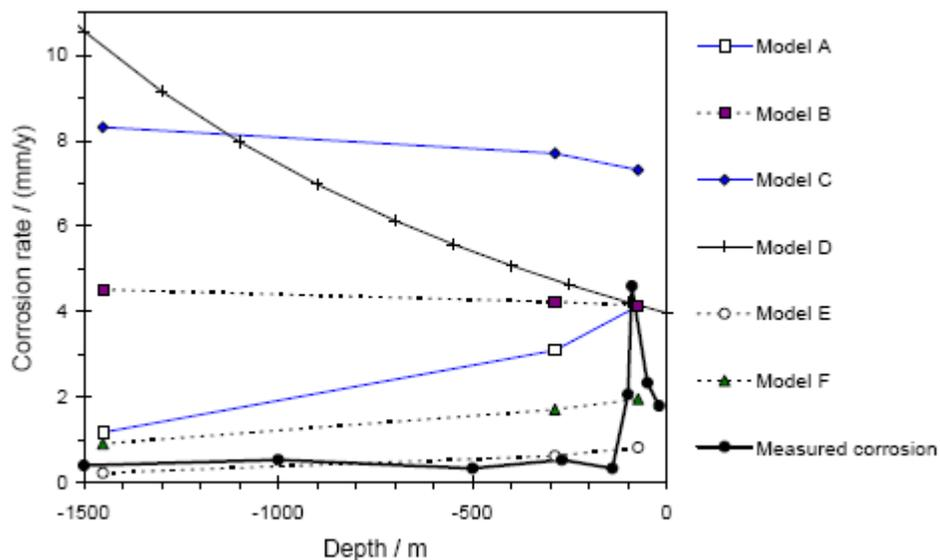
Figure 2.2.1: Predicted and measured corrosion rates at different depths in Oil well.
