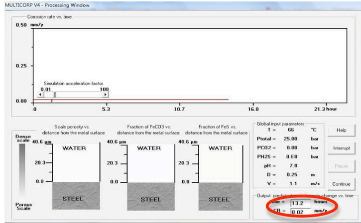
Figure 4.2.2.2: Operation stage MULTICORP.
