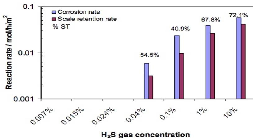
Figure 2.2.5: The comparison of corrosion rate (CR) and scale retention rate (SRR) in the same molar units as a function of H<sub>2</sub>S gas concentration.
