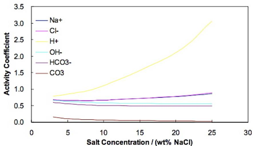
Figure 2.2.4: Calculated activity coefficient change with salt concentration at 20°C at 1 bar total pressure.
