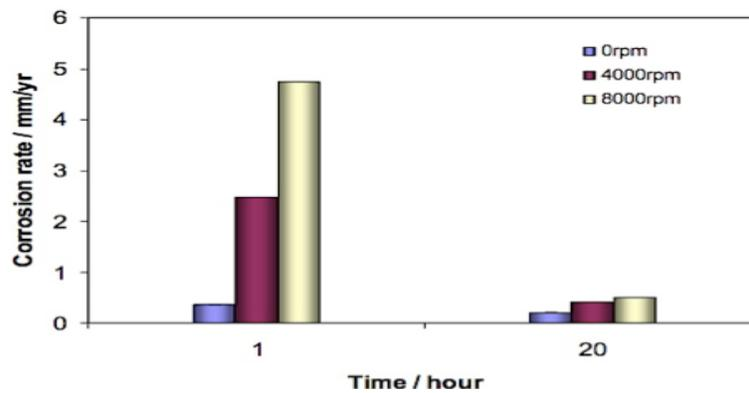
Figure 2.2.7: The corrosion rate vs. time for different rotational speeds.
