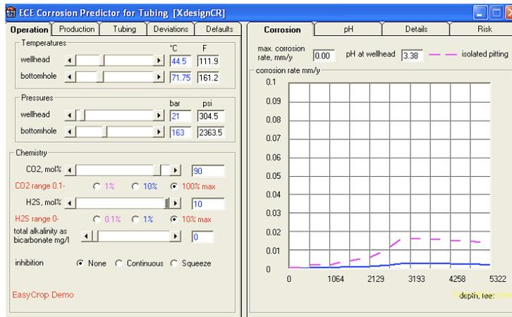
Figure 4.2.1.6: Presence of H<sub>2</sub>S reduces corrosion rate.
