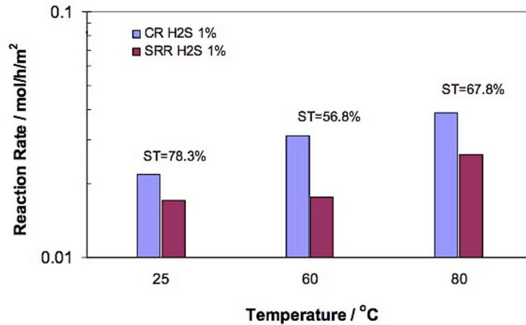
Figure 2.2.6: The corrosion rate (CR) and scale retention rate (SRR) vs. temperature.
