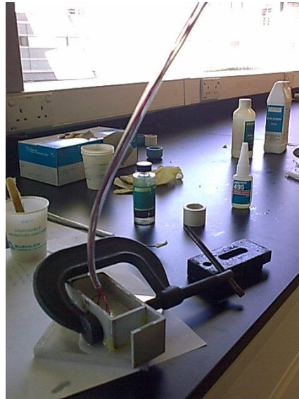
Figure 13: Set-up for Cold Mounting
