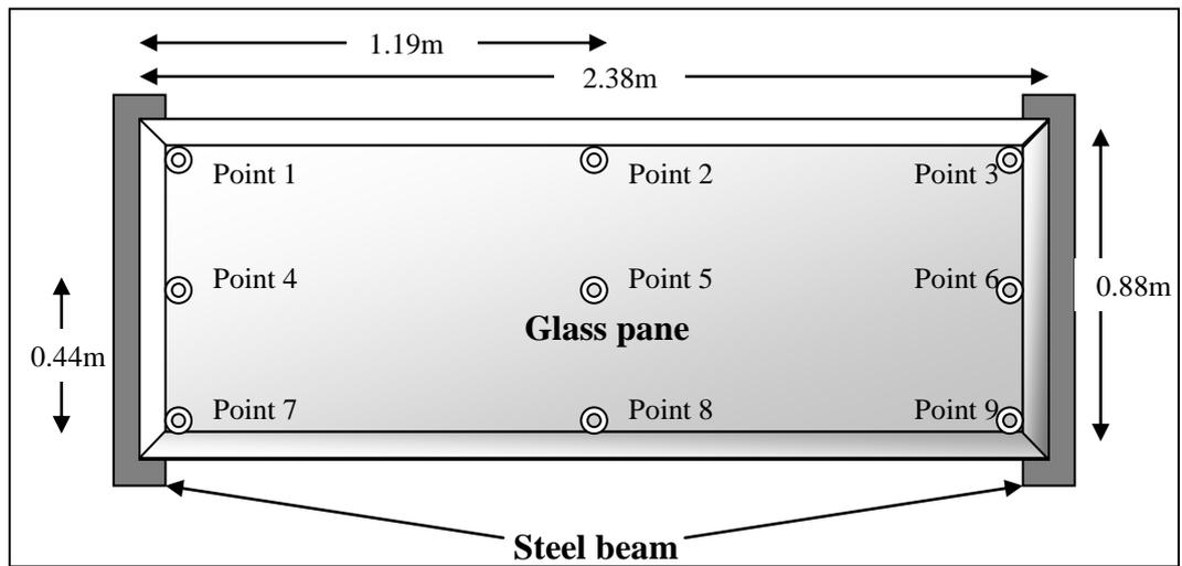
Figure 4.11: Schematic diagram of the glass pane
