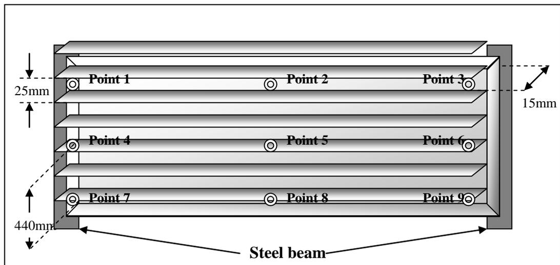
Figure 4.14 : Schematic diagram of the experiment
