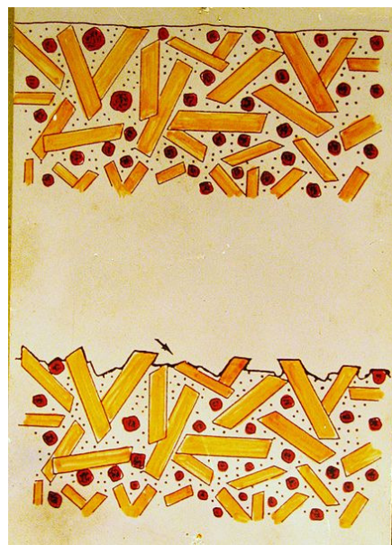
Figure 2.3.8: Diagram showing paint pigments in a resin matrix. It can be seen that weathering only removes the smaller pigments, resulting in the color change [17]
