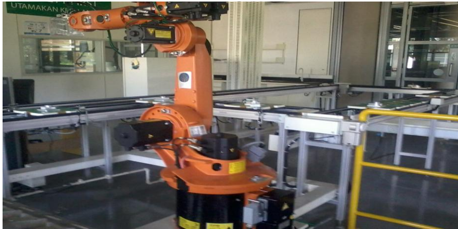
Figure 11 Robotic Arm Gripper (armKuka K15)
