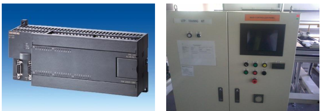
Figure 16 LEFT: SIEMENS PLC S7-200 RIGHT: PLC Cabinet
