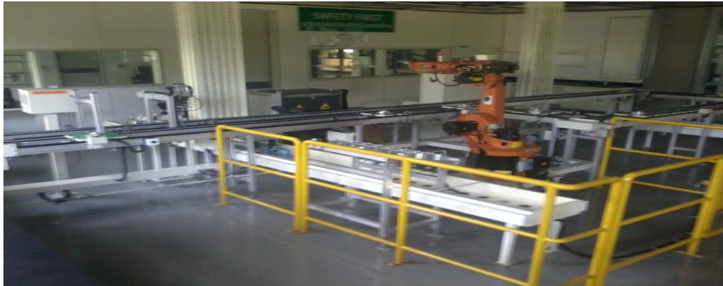
Figure 8 PLC- Controlled Conveyor System in UTP lab
