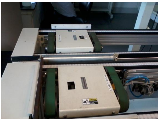
Figure 23 LEFT: DIVERTER STUCK WHEN PALLET REMOVE RIGHT: CLOSE PALLET DISTANCE
