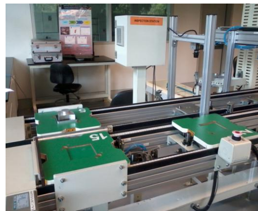
Figure 23 LEFT: DIVERTER STUCK WHEN PALLET REMOVE RIGHT: CLOSE PALLET DISTANCE
