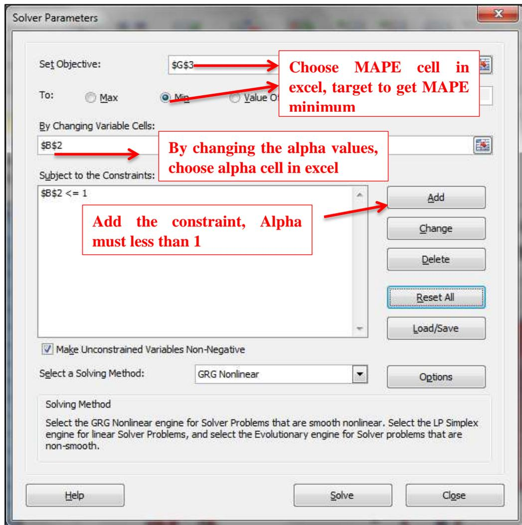
Figure 4 Solver Parameter Plugin
