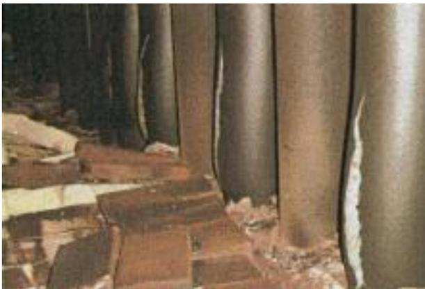
Figure 2: Photograph of failed tubes
