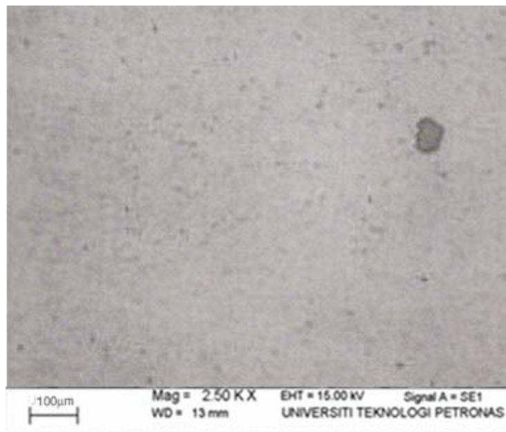
Figure 17: Largest Oxide Inclusion of Steel Sample A2
