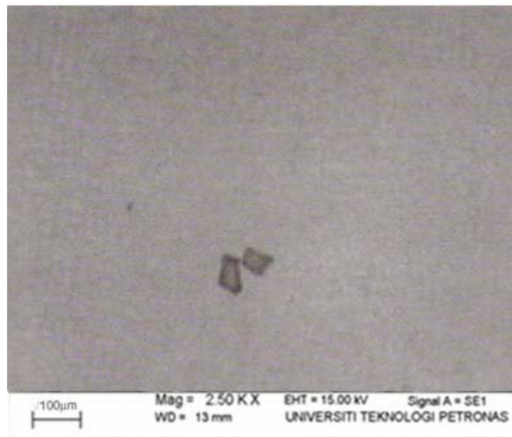
Figure 16: Largest Oxide Inclusion of Steel Sample A1
