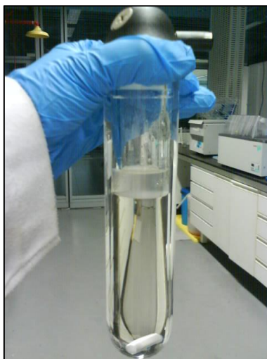
Figure 14 : Two layers of anion and unreacted materials
