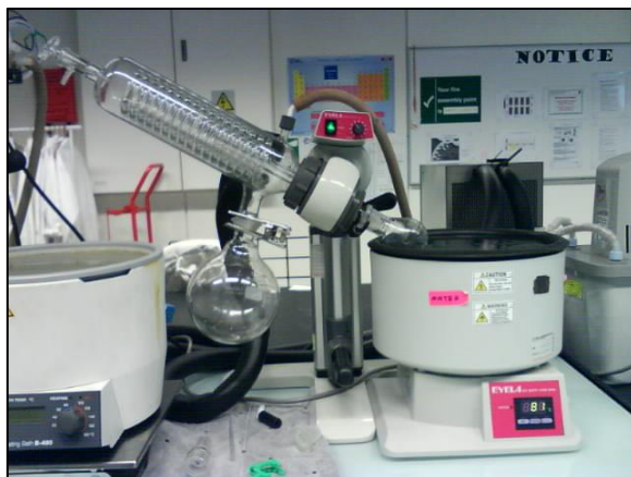
Figure 15 : Removal of ethyl acetate and unreacted material by rotary evaporator
