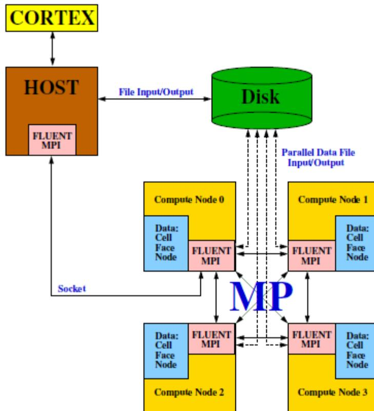
Figure 5: Parallel Ansys Fluent Architecture
