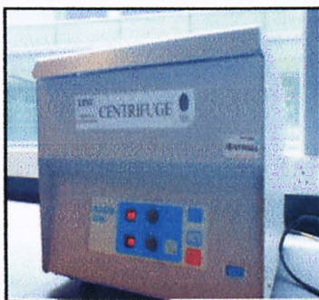
Figure D.2: Separation of [BMIM][DBP] ionic liquid and model oil using centrifuge.
