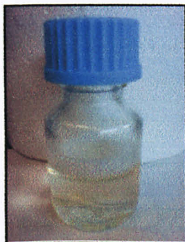
Figure C.1: Mixture of 10ml of model oil and 1ml of Hydrogen Peroxide after oxidation
