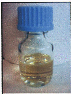
Figure C.1: Mixture of 10ml of model oil and 1ml of Hydrogen Peroxide before oxidation.
