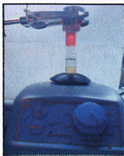
Figure 3.4: Mixing process using vortex mixture.
