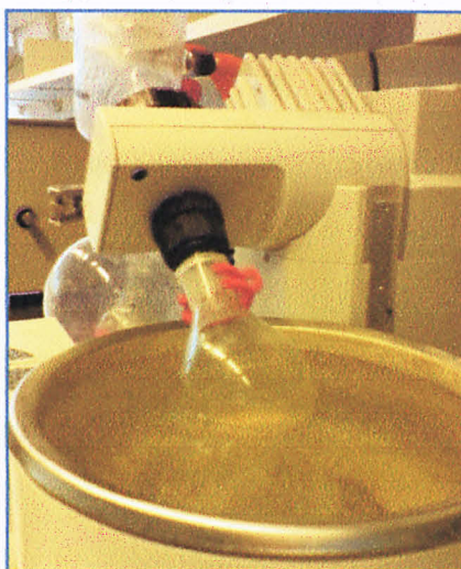
Figure A.3: Rotary evaporation process to remove residual.
