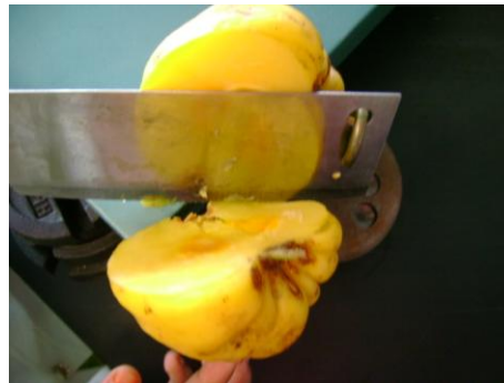
Figure 4.6: Stop increased the load when the fruit is fully cut. The final load is 60 N.
