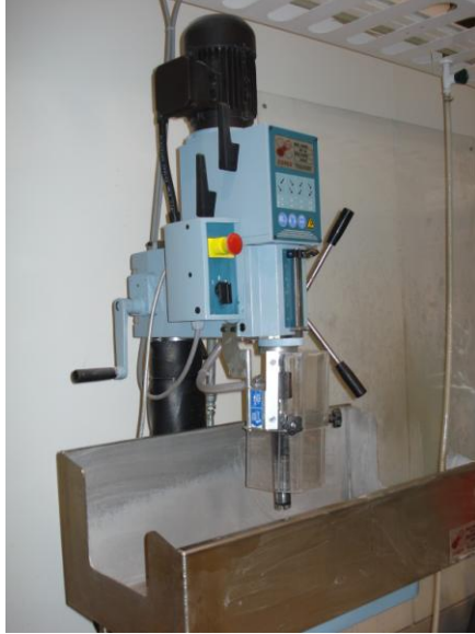
Fig 4: Core 1 is being reduced in diameter by Coring Machine
