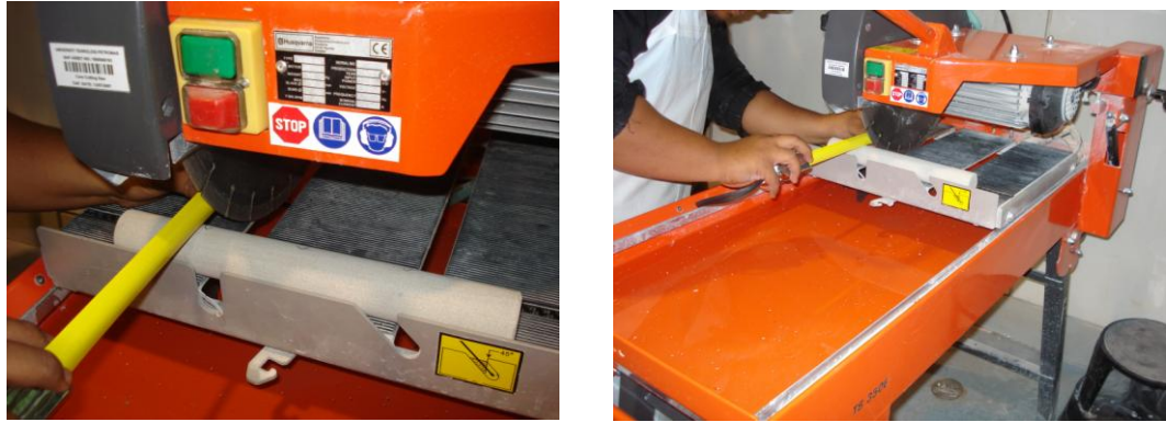
Fig 2: Core 2 is cut using Cutting Saw Machine
