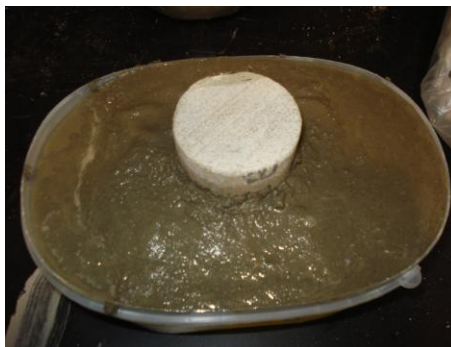
Fig 1: Core 1 is cemented in transparent container
