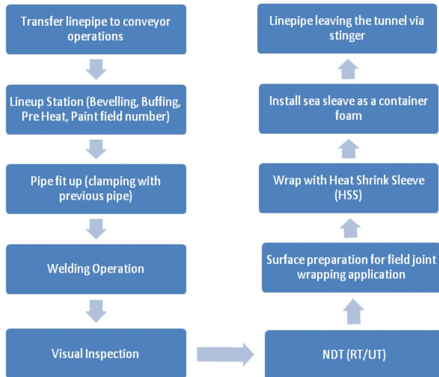
**Fig 2.2: S-Lay Linepipe Installation Process**
