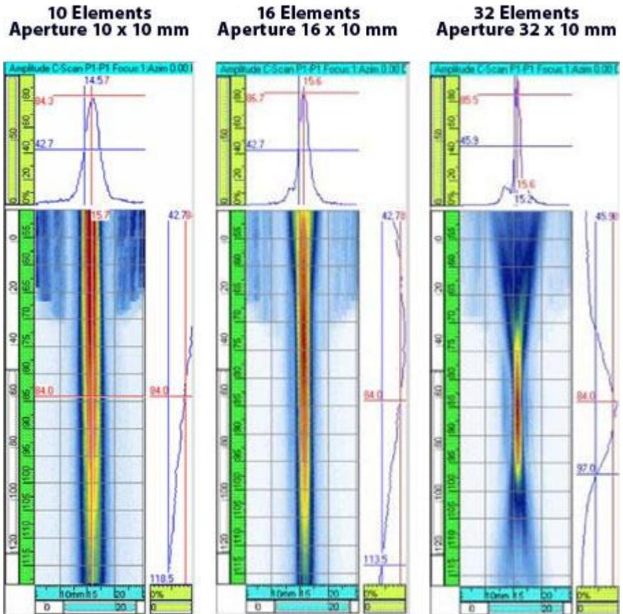
**Fig 2.27: Difference between the elements and aperture**
