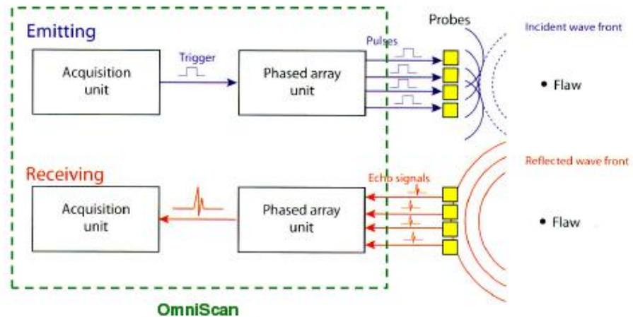
**Fig 2.16: The reflection pulse detected and receives in an echo signals (sine waves)**
