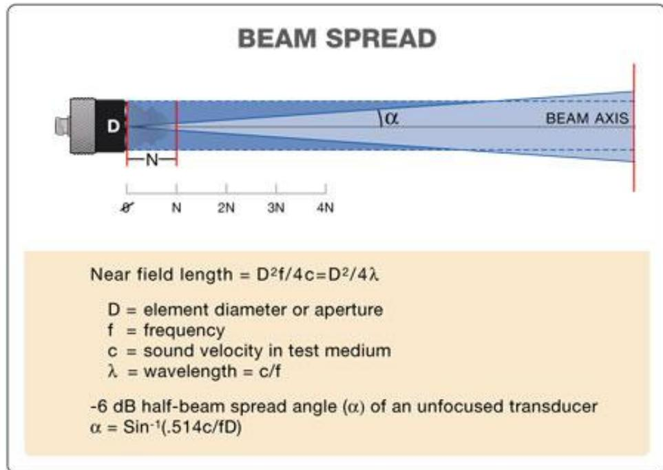
**Fig 2.3: Beam Spread equation to find the Near Field Length**
