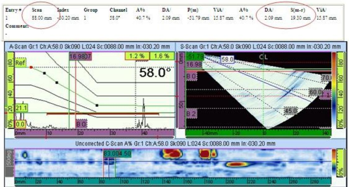
**Fig 4.9: Result for the 1<sup>st</sup> crack. Inside the red circle, DA indicates the depth and S(m-r) indicates the length of the crack. The scan is the location of the crack.**
