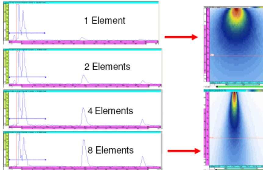
**Fig 2.18: The number of elements provides the focal point of the image**
