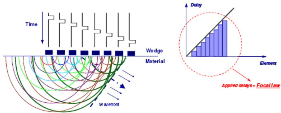
**Fig 2.15: The element control the wave front**
