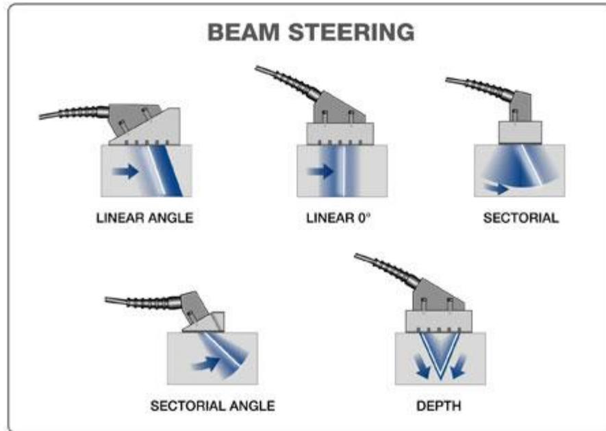
**Fig 2.21: Type of beam steering**
