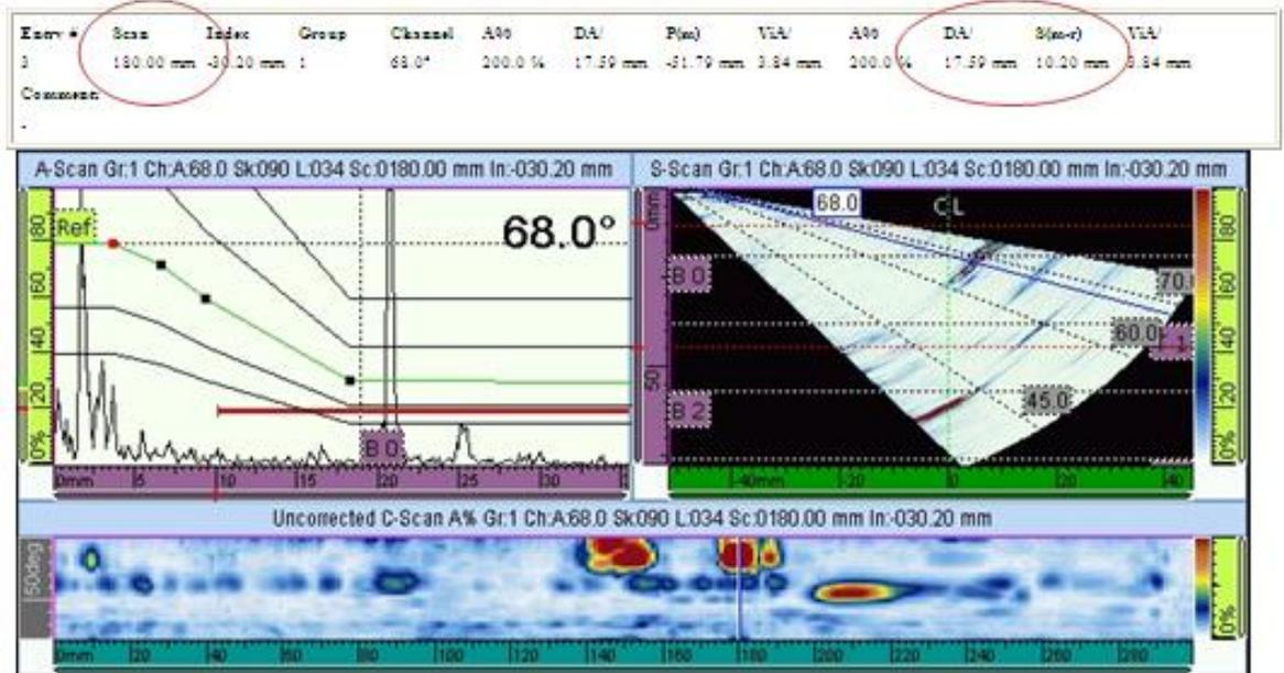
Fig 4.11: Result for the 3<sup>rd</sup> crack
