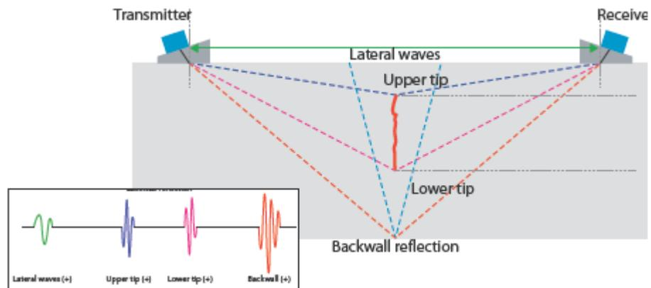
Fig 4.3: ToFD Principle
