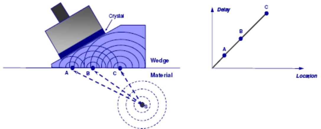
**Fig 2.14: The reflection waves gives a signal back to the probe and detected by the crystal**
