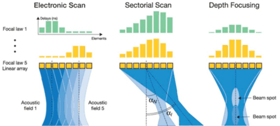
**Fig 2.20: Concept for generation of linear and sectorial scans using phased arrays**
