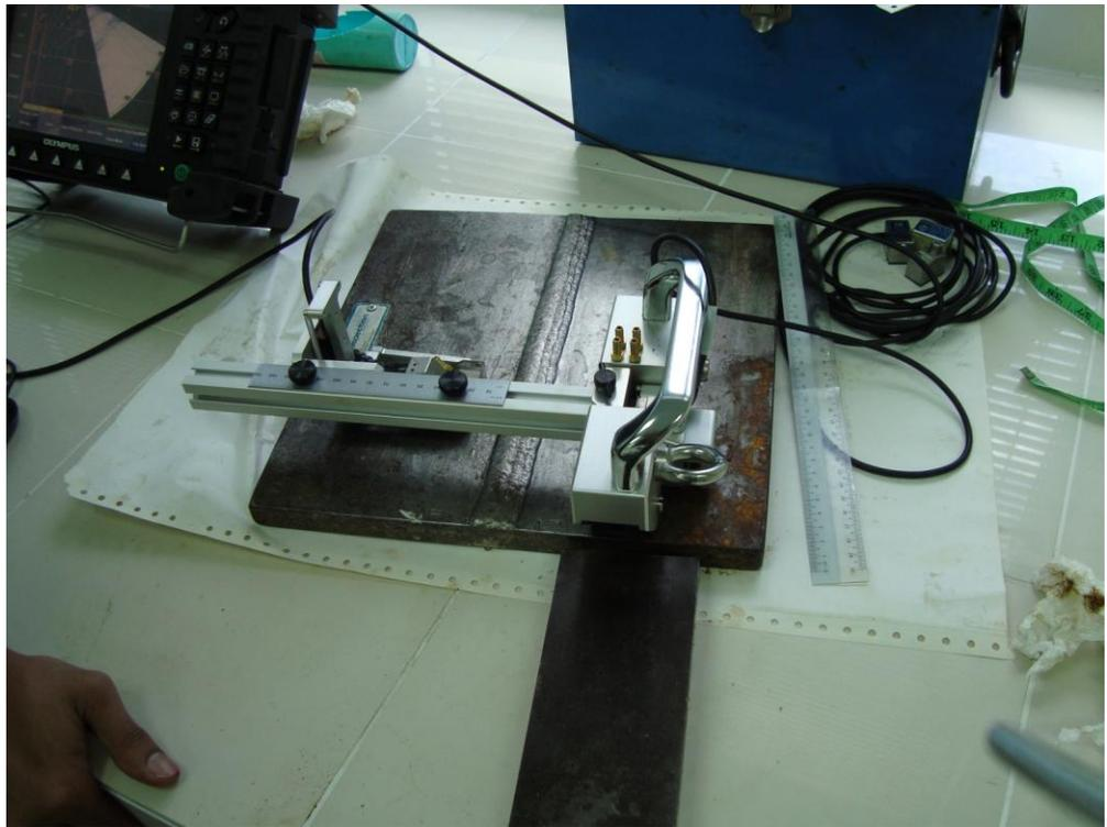
**Fig 4.5: Phased Array with the decoder to measure the distance travel for accuracy**
