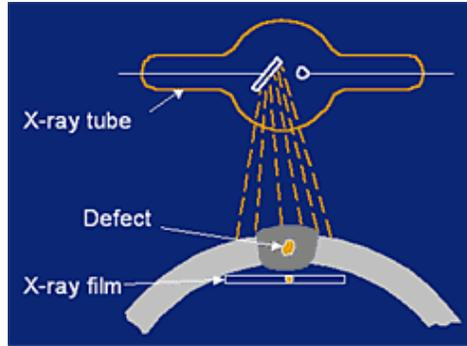
**Fig 1.3: Radiographic Inspection**
