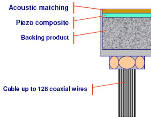
**Fig 2.19: Piezo composite probe consists up to 128 elements**
