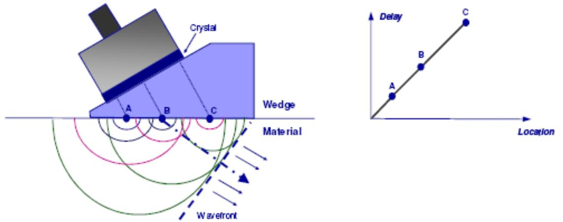
**Fig 2.13: The delay control the angle of wavefront**
