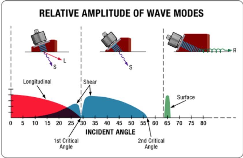
**Fig 2.7: Relative Amplitude of Wave Modes (Longitudinal, Shear and Surface Waves)**
