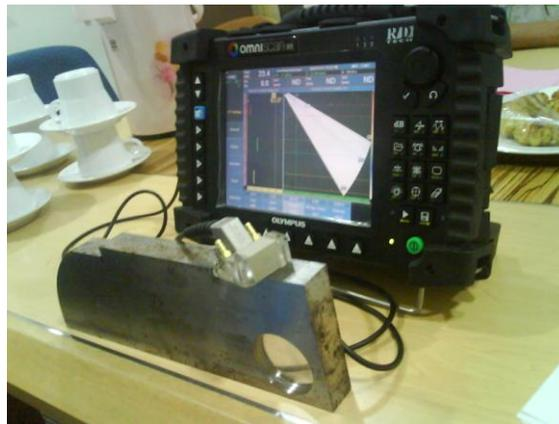
Fig 2.9: PA machine with a probe on a calibration block
