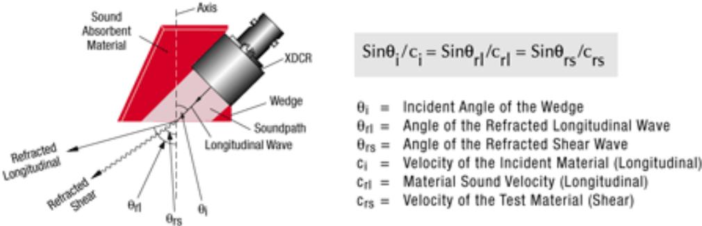
**Fig 2.6: Equation to find the incident angle**
