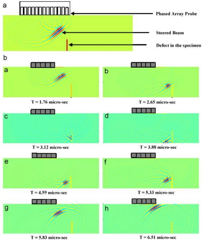
**Fig. 2.10: Beam steering and focusing in a phased array transducer. (b) Interaction of a phase steered wave with the crack tip and corner.**
