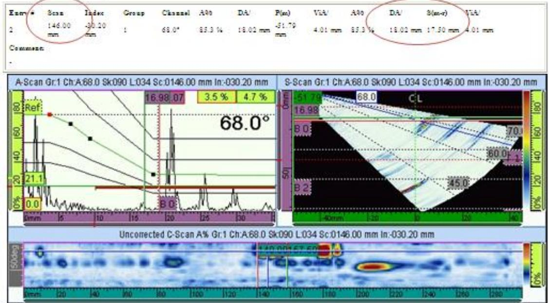
Fig 4.10: Result for the 2<sup>nd</sup> crack
