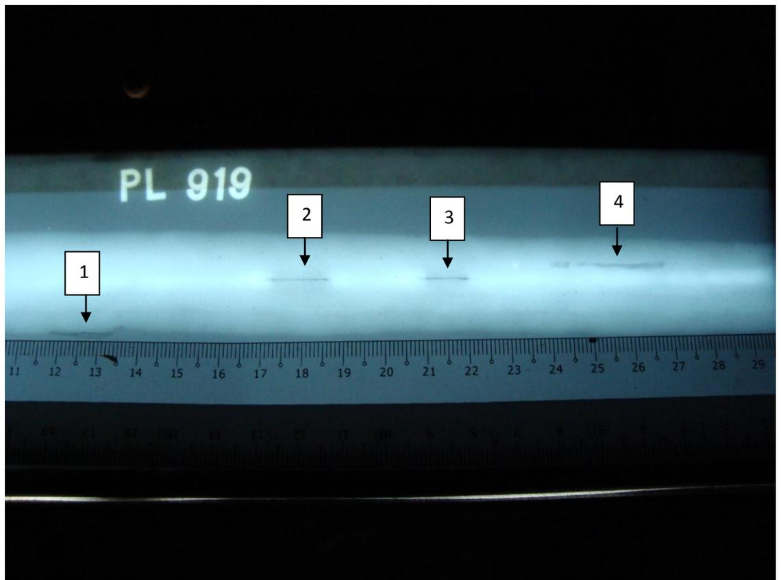
**Fig 4.8: It indicates that there are 4 cracks at the weldment**
