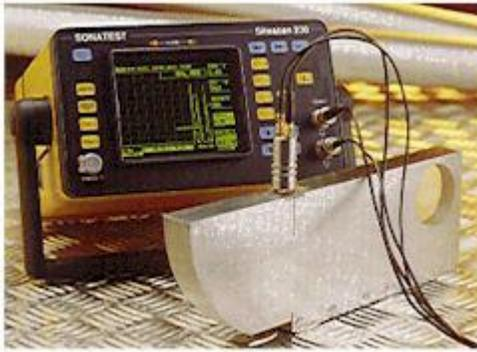
**Fig 1.1: Ultrasonic Equipment**
