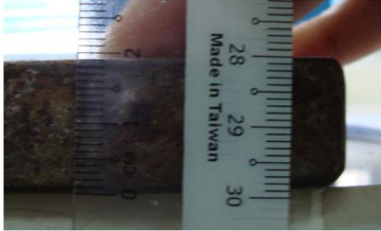
**Fig 4.6: Thickness of the plate (19mm)**
