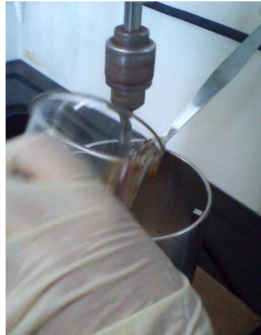
Figure 3.4: mixing HA latex, H 2 O, SiO 2 and RWL
