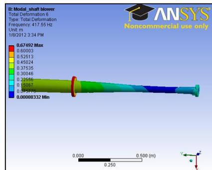
Figure 4.4: Deformation at 75Hz
