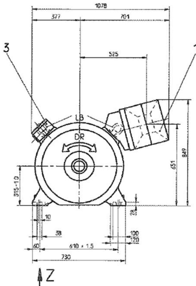
Figure 3.2: Dimension of motor [4]
