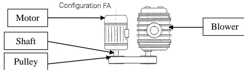
Figure 1.3: Main components of blower unit [4]
