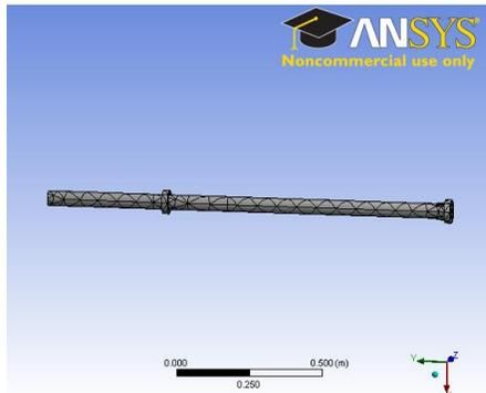
Figure 3.4: Mesh model of blower's shaft
