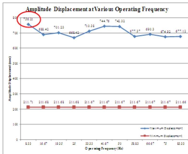
Figure 4.1: Amplitude response at difference operating frequency
