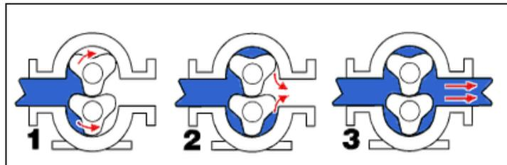
Figure 1.2: Working principle of blower [3]
