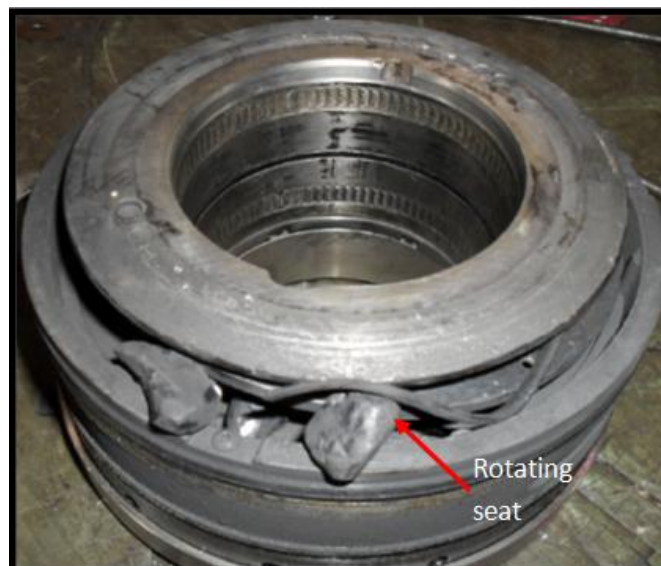
Figure 2.6: Dry gas seal damage due to surging (PETRONAS, 2010)
