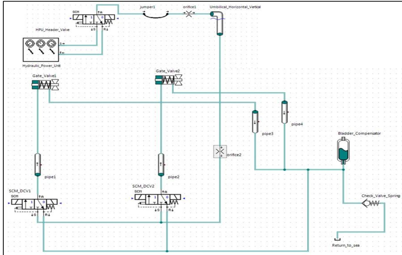
Figure 4-2: Subsea Control Module model in Agito SimulationX
