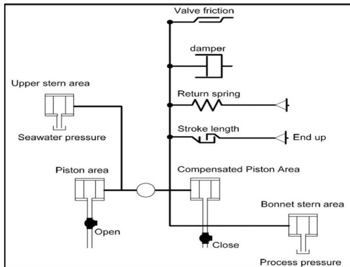
Figure 3-6: Gate Valve model. (SimulationX, 2008)
