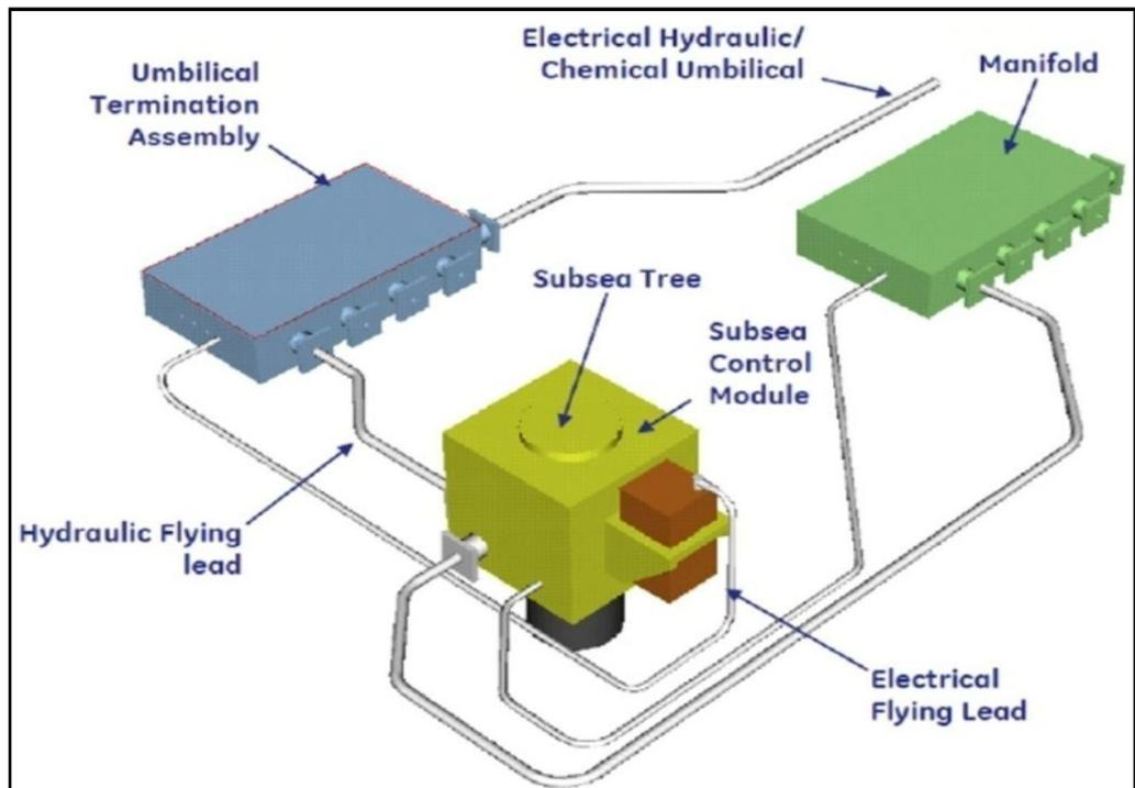
Figure 2-2: Subsea production system subsea facilities. (Yong, 2010)
