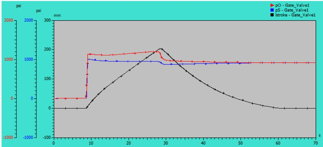
Figure 5-3: Effect of 7 inch valve size on response.
