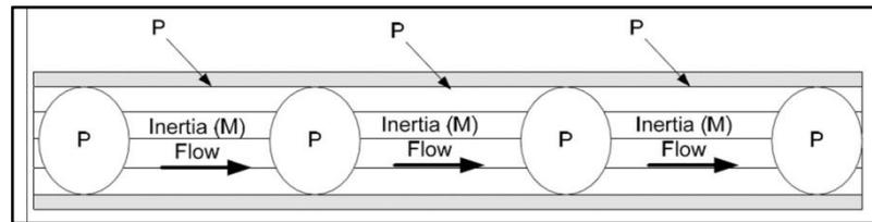
Figure 3-4: Distributed line model. (SimulationX, 2008)
