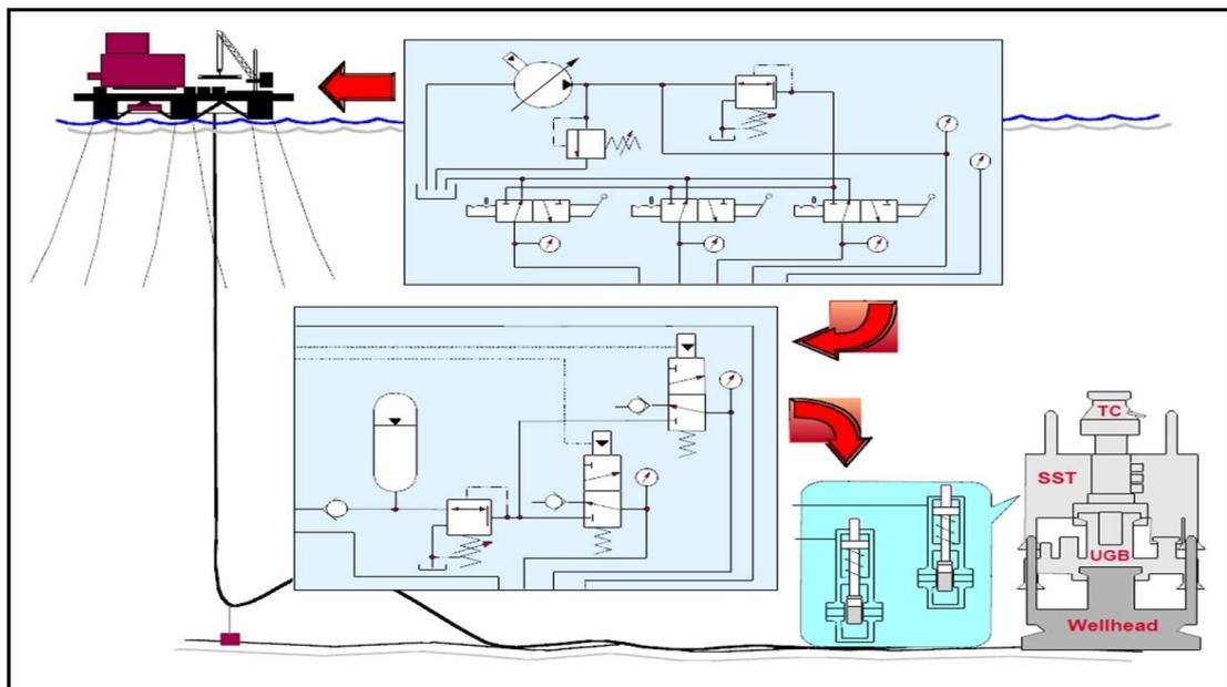
Figure 2-3: Piloted Hydraulic Control System. (Stecki, 1998)
