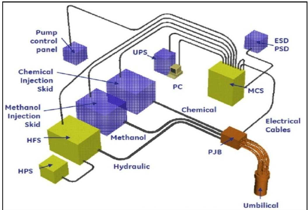
Figure 2-1: Subsea production system topside facilities. (Yong, 2010)
