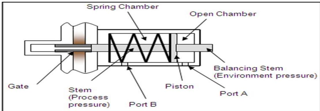
Figure 2-5 : Gate Valve principal drawing. (SimulationX, 2008)
