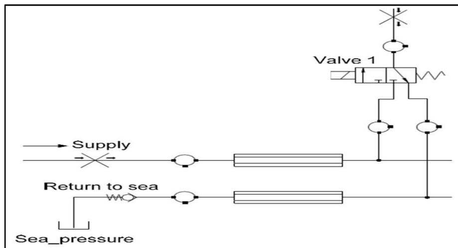
Figure 3-5: Subsea Control Module model. (SimulationX, 2008)
