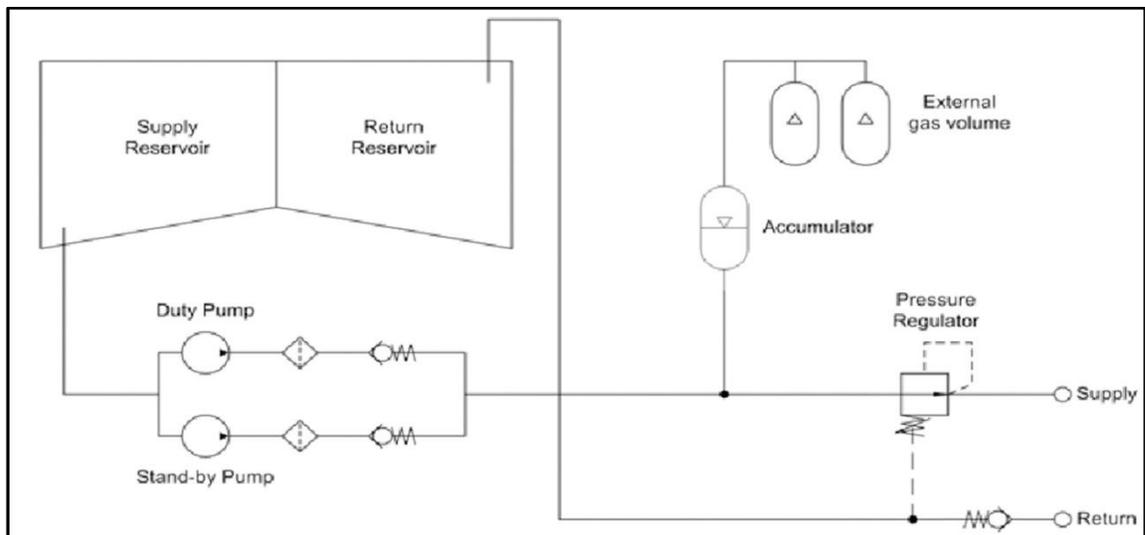
Figure 3-3: Hydraulic Power Unit model block diagram. (SimulationX, 2008)
