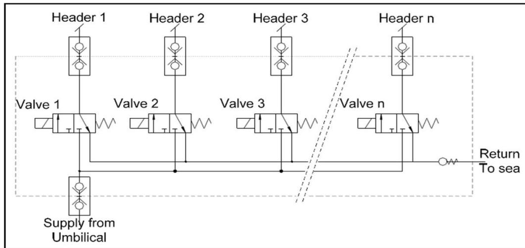
Figure 2-4: Schematic diagram of Subsea Control Module. (Agito, 2008)
