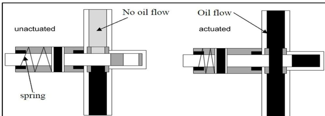
Figure 2-6: Gate Valve in Close and Open positions. (SimulationX, 2008)
