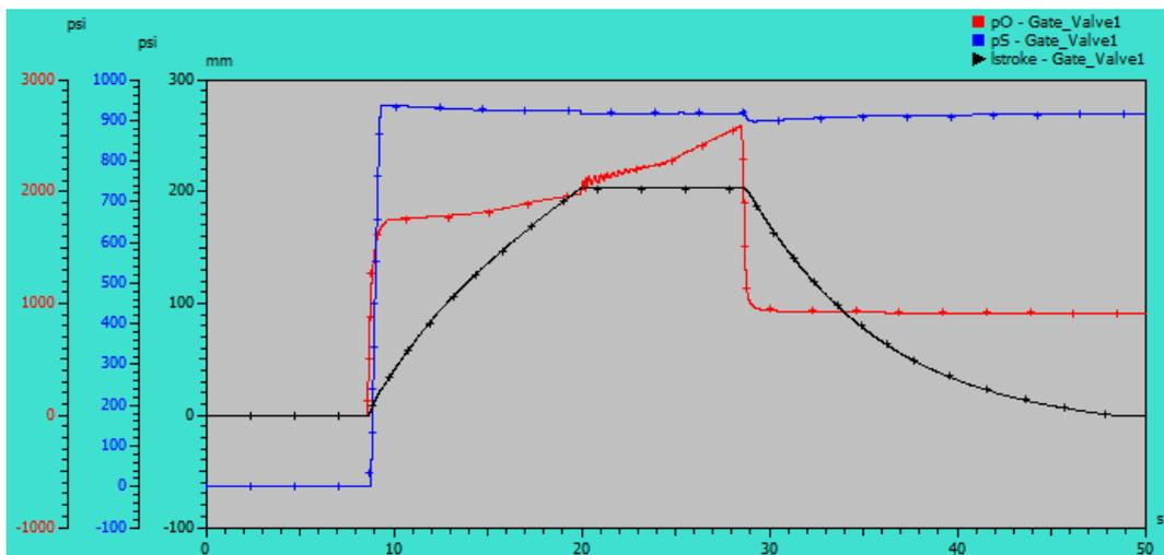
Figure 5-1: Effect of valve movement on response time.
