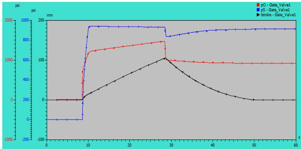
Figure 5-2: Effect 1/4 inch hose size on response time.
