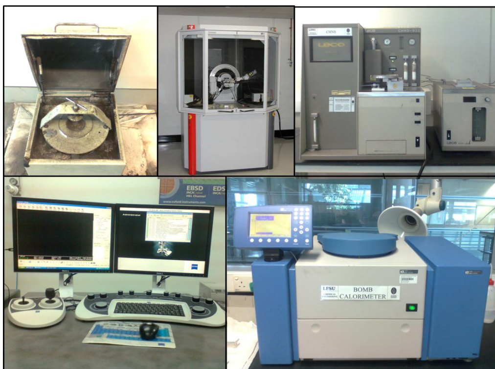
Figure 3.2: From top left, counter clockwise - Mortar Grinder, FESEM-EDS, Bomb Calorimeter, CHNS Analyzer, XRD equipment.
