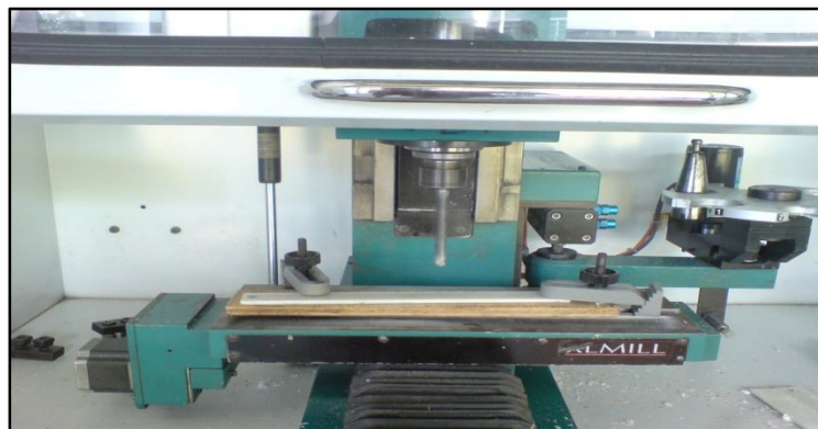
Figure 3.5: Drilling of GFRE samples
