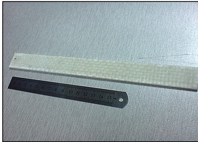
Figure 3.4: GFRE sample (250x50 mm)
