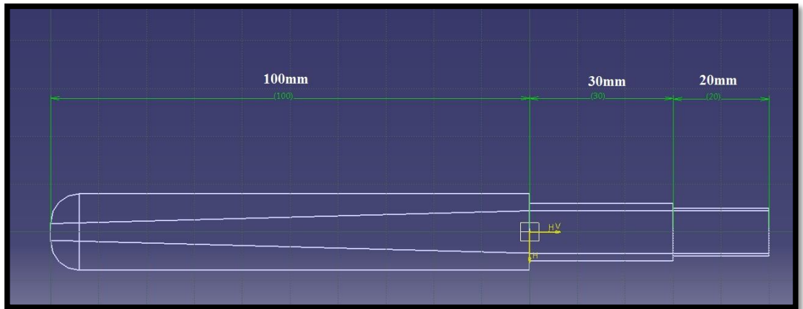
Figure 4.8: Side view of the nozzle dimension (units in mm)
